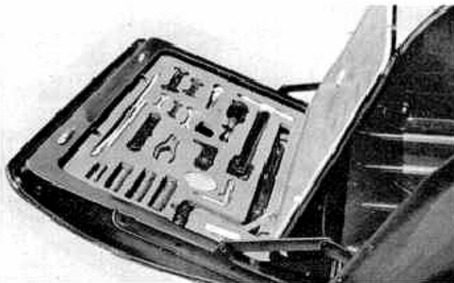
Only a British car of quality provides such examples as this tool tray on the Jaguar of close attention to the owner's personal convenience. There is a light in the lid for illumination at night.
