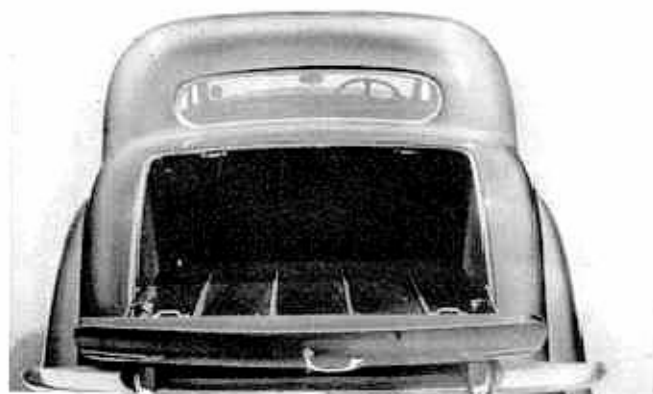
The luggage compartment interior is unusually well finished, and has rubber inset strips for protection. Spare wheel and wheel-changing tools are in a separate compartment below.
