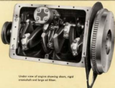
Under view of engine showing sump, rigid crankshaft and large oil filter.
