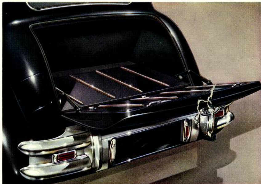
The capacious luggage compartment is fitted with rubber protector strips, the lid forming a platform for additional luggage. Tools are carried in the lid (see page 8).
