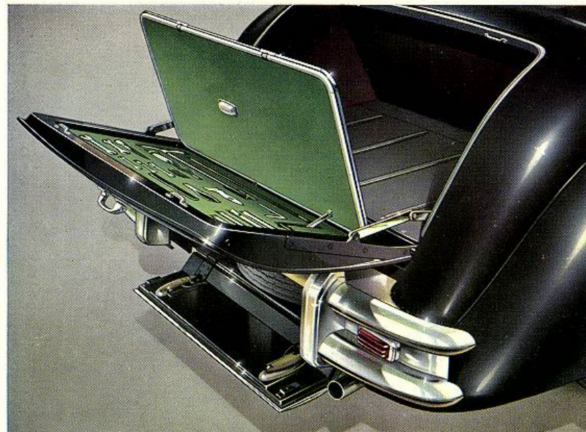
Tools are carried in special soundproof container fitted with automatically controlled light.
