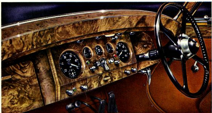
Instrument panels of all closed models are of seasoned wood with polished figured walnut finish. The glove drawer at the bottom centre can be removed to accommodate wireless control panel.
