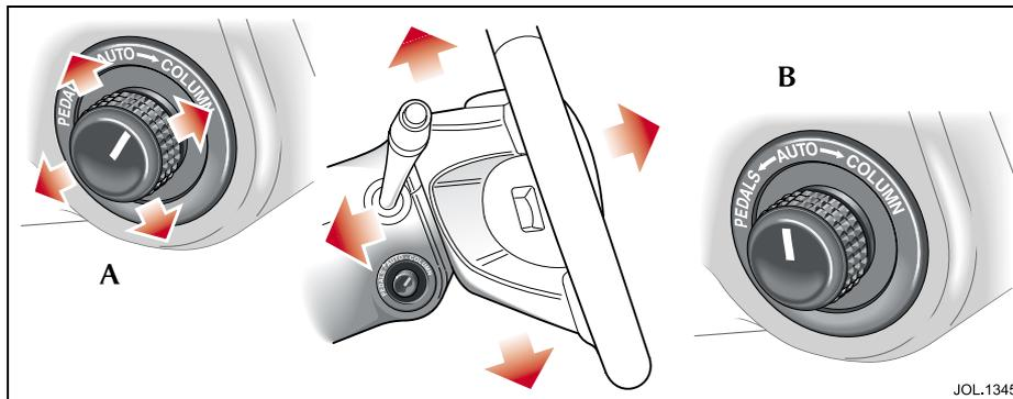
**Exit** – If the ignition key is in position '0' and the driver's door is opened or if the ignition key is removed, the steering column will move to the uppermost tilt position and the seat will move slightly rearwards.
