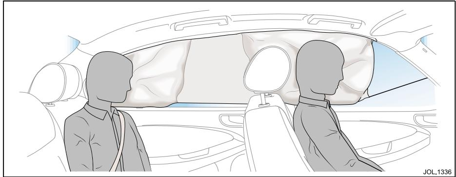
The curtain airbag on the front passenger side is always deployed in a side impact even if the front passenger seat airbags are de-activated. This is to maintain protection for a rear occupant.
