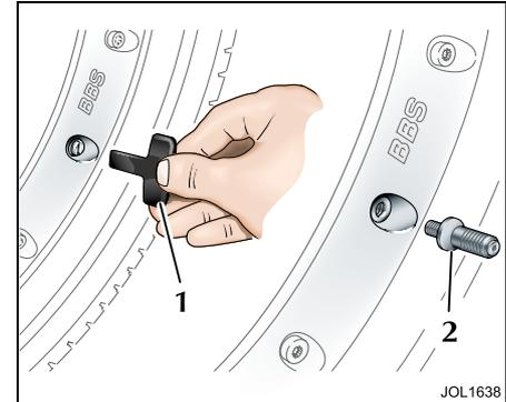
**'R' performance wheels** – These wheels have a slotted screw valve cover on the wheel face. A pouch containing a 'T'-shaped screwdriver and a valve adaptor, for use with these wheels, is stowed in the glove compartment.
