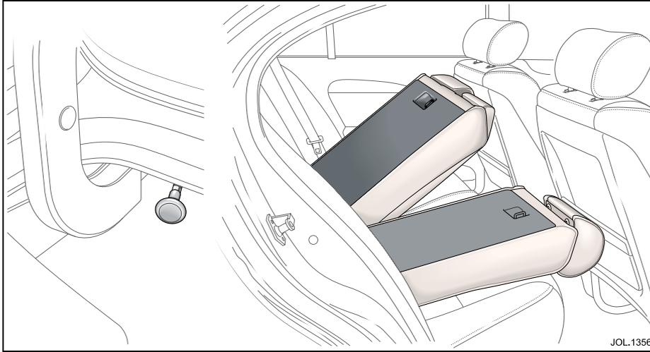
Ensure when folding the seat back down that the armrest is stowed and that there is sufficient clearance between the seat back, including the headrest, and the back of the front seat.
