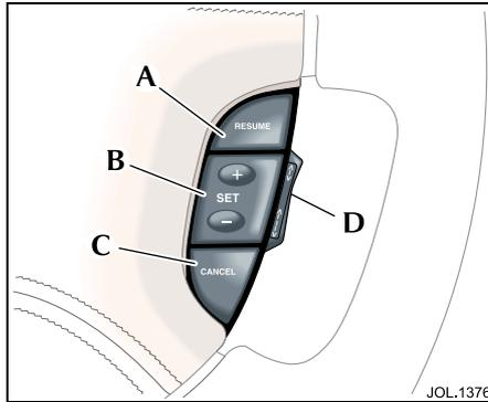
The system is operated by switches mounted on the steering wheel. The driver can also intervene at any time by use of the brake or accelerator pedals. The steering wheel switches operate as follows:
