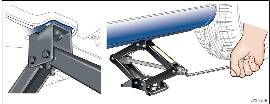
Before raising the vehicle slacken but do not remove the wheel nuts.
