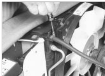
5.3 Remove the clamp and the hose going to the expansion tank
