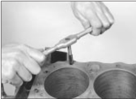
15.8 All bolt holes in the engine block - particularly the main bearing cap and cylinder head bolt holes - should be cleaned and restored with a tap (remove debris from holes after this is done)
