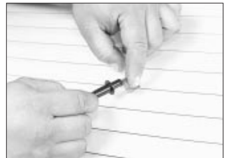
16.4 When measuring the voltage at the heated rear window grid, wrap a piece of aluminium foil around the negative probe of the voltmeter and press the foil against the element with your finger
