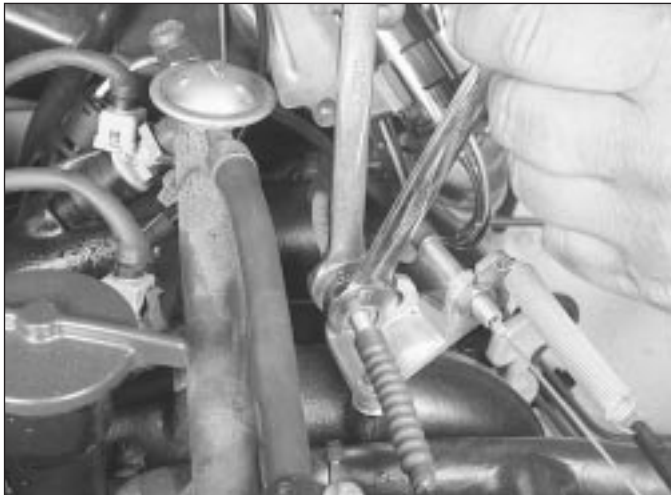
10.2 Loosen the locknuts on the accelerator cable
