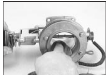
13.18 The area inside the throttle body near the throttle plate suffers from sludge build-up because the PCV hose vents crankcase vapour into the intake duct
