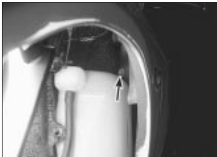
15.7d Remove the wing-to-door pillar bolt (arrow; lower bolt not visible)
