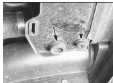
5.8 There are rubber mounts (arrowed) for the radiator and the condenser - they must be in place when these components are reinstalled
