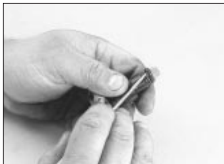
13.38a If you plan to refit the original injectors, remove and discard the O-rings and grommets and fit new ones
