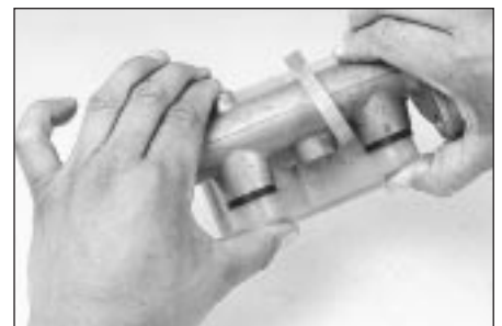
6.7t . . . and squeeze the reservoir and master cylinder together; make sure the reservoir is fully seated
