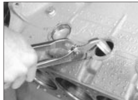
15.1b Pull the core plugs from the engine block with pliers
