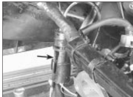
15.4a Disconnect the solenoid electrical connector at the harness connector located near the bulkhead behind the cylinder head (arrowed)
