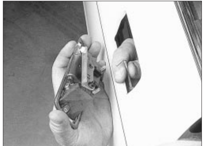
20.8 Detach the plastic clip securing the lock rod
