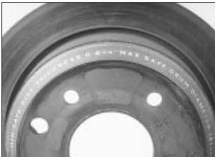
5.5b Compare your measurement with the minimum thickness stamped into the disc
