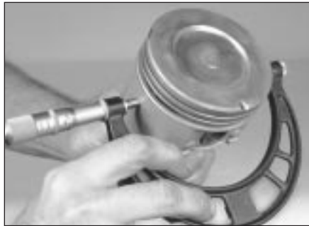
18.11 Measure the piston diameter at a 90° angle to the piston pin, at the bottom of the piston pin area - a precision caliper may be used if a micrometer isn't available
