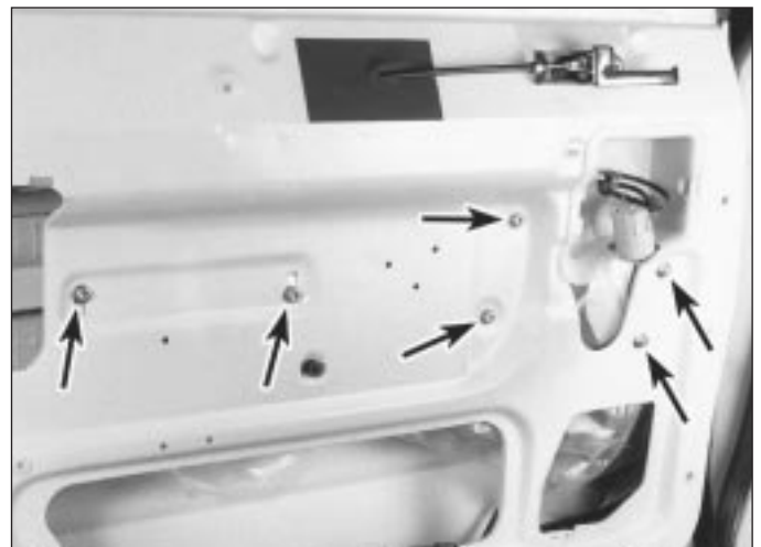
21.3 Detach the window regulator bolts (arrowed)
