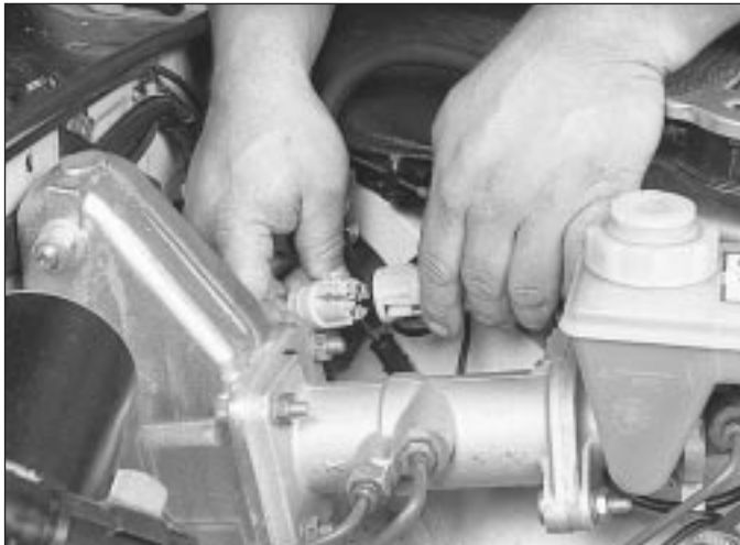
6.4 Trace the electrical lead back from the reservoir cap and disconnect the low fluid level sensor
