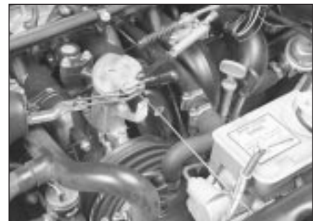
10.10 Attach a strong wire (coat hanger) to the master cylinder using a clamp and align it with the notch on the bellcrank
