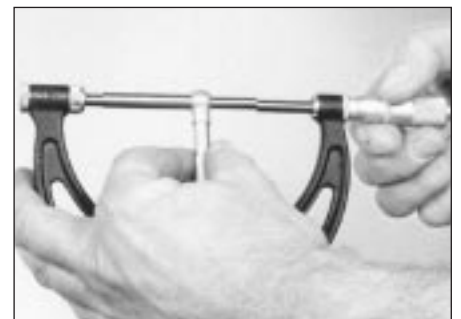
16.4c The gauge is then measured with a micrometer to determine the bore size
