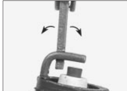
4.4b To change the gap, bend the side electrode only, as indicated by the arrows, and be very careful not to crack or chip the porcelain insulator surrounding the centre electrode
