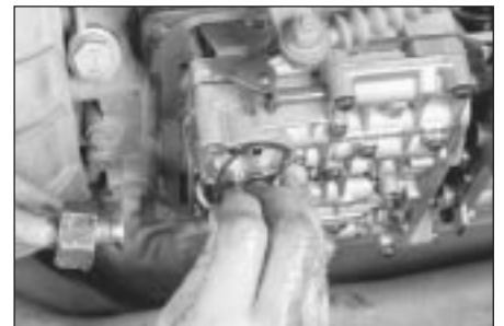
26.10c Be sure to remove the old O-ring from the transmission - always use a new O-ring when replacing the filter
