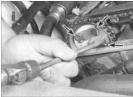
10.12 Bend back the locking tabs (arrowed) and remove the camshaft sprocket bolts
