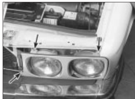
17.3a Remove the two retaining screws at the top and the one in the grille opening (arrowed)
