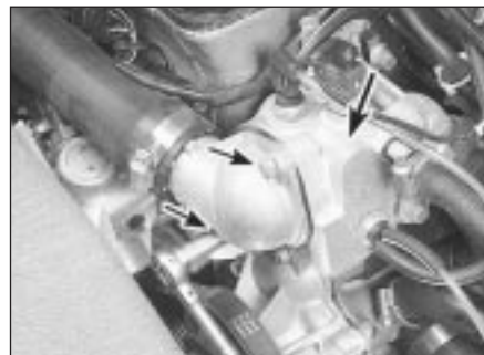
3.7 Remove the two bolts (small arrows) holding the thermostat cover to the housing (large arrow)
