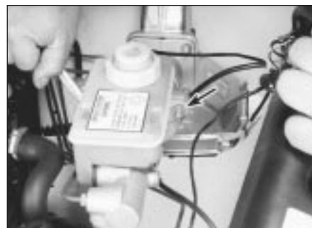
6.6 Remove the two master cylinder mounting nuts
