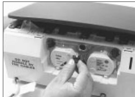
21.10 To remove an instrument cluster bulb, depress the bulbholder and rotate it anti-clockwise
