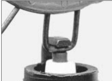
4.4a Spark plug manufacturers recommend using a wire-type gauge when checking the gap - if the wire does not slide between the electrodes with a slight drag, adjustment is required
