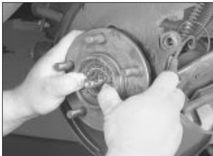
22.20 Refit the hub assembly onto the spindle - then push the grease-packed outer bearing into position
