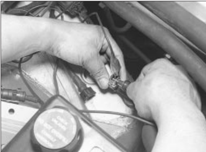
4.13 To test the oxygen sensor heater, disconnect the electrical connector, and working on the sensor side, check the resistance across the two terminals. Heater resistance should be 5 to 6 ohms
