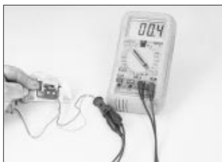
13.7b With the switch plunger depressed, there should be continuity (zero resistance)
