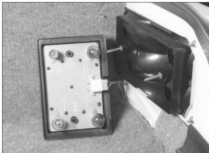
21.5 Remove the bulb cluster from the tail light housing - The bulb is removed by pushing in and turning the bulb anti-clockwise
