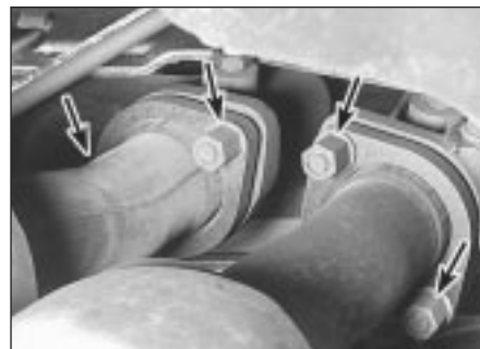
14.4 Use penetrating spray on the exhaust flange nuts before attempting to remove them
