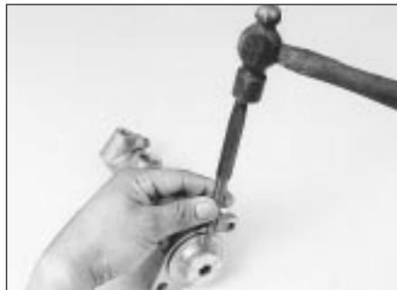
6.7q Using a hammer and punch, stake the end plate as shown (there's a dimple in the side of the plate for this purpose)
