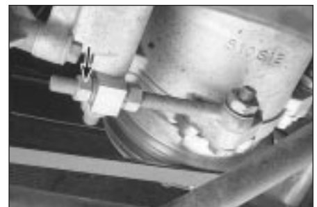
21.6b To adjust the air conditioning compressor drivebelt, loosen the outer locknut (arrowed) and the compressor pivot bolts - turn the inner locknut anti-clockwise to loosen or clockwise to tighten the belt
