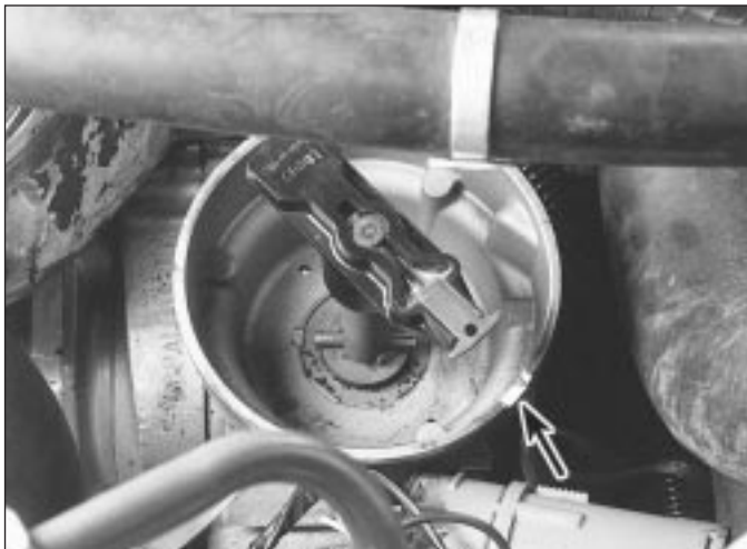
9.5a Paint or scribe a mark (arrowed) on the edge of the distributor housing below the rotor tip to ensure that the rotor is pointing in the same direction when the distributor is reinstalled
