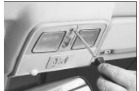
24.13 Remove the plastic screw, then pull the overhead console down and unplug the electrical connectors
