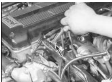
5.7a Remove the ground strap from the front stud (arrowed), and the engine wiring harness clips from the other studs
