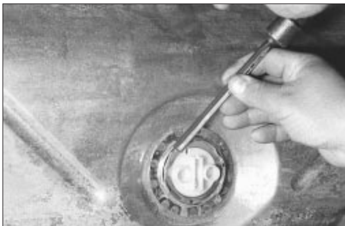
5.10 Use a brass punch and remove the lock ring by tapping on it in an anti-clockwise direction
