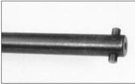
8.2a When refitting the spring compressor tool (JD115), insert the upper end of the rod into the cross-shaped slot in the suspension crossmember, then rotate the rod 90° so this pin on the upper end of the tool locks into the crossmember
