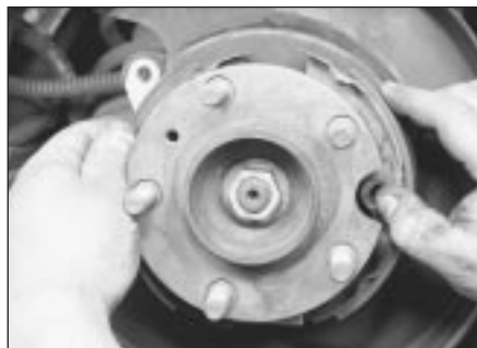
12.5e Push the shoes together and disengage the upper return spring from the rear shoe . . .
