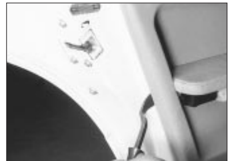
18.9 Disengage the retaining clips along the outer edge of the door trim panel
