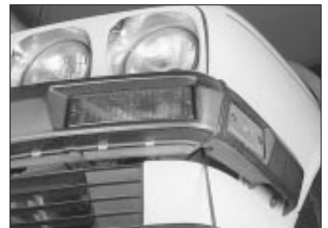
17.3b The retaining screw at the outside lower corner can be accessed from under the bumper
