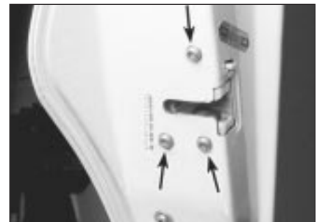
20.4 Remove the latch screws (arrowed) from the end of the door, and pull the latch assembly through the access hole.
