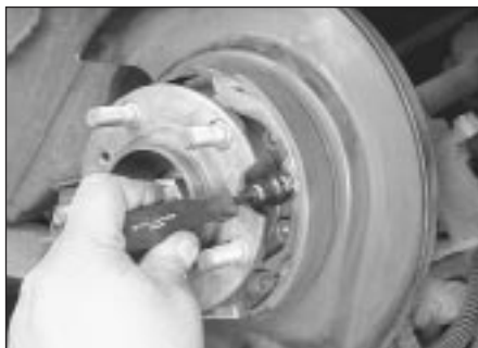
12.5d Remove the rear hold-down spring, washers and pin; put the parts in a plastic bag so you don't lose them
