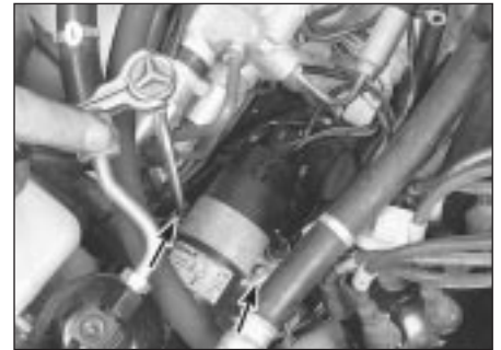
8.7 Remove the nuts from the coil mounting bracket (arrowed)
