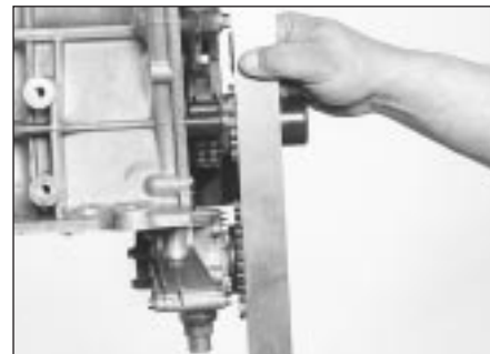
13.18 Check the oil pump and crankshaft sprocket alignment with a straightedge - add or subtract shims until the sprockets are aligned for smooth chain operation
