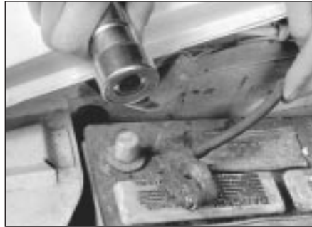
6.7b Regardless of the type of tool used to clean the battery posts, a clean, shiny surface should be the result
