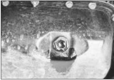
Engine oil may leak from the drain plug...
