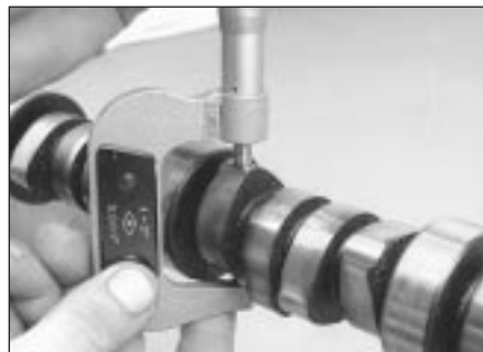
10.21a Measure the camshaft lobe at its greatest dimension . . .
