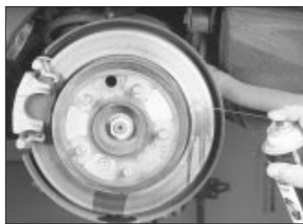
3.5a Before starting, wash down the caliper and disc with brake cleaner
