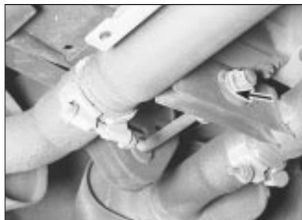
14.1c On dual silencer models, check the condition of the mount (arrowed) and the clamps
