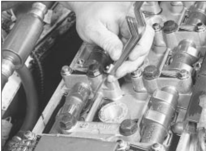
10.4 Measure the valve clearance with a feeler gauge inserted between the heel of the camshaft lobe and the lifter
