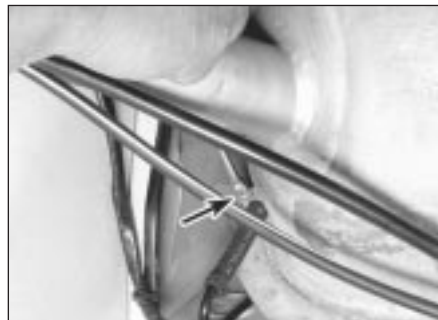
7.9c Disconnect the canister purge line from the fuel tank
