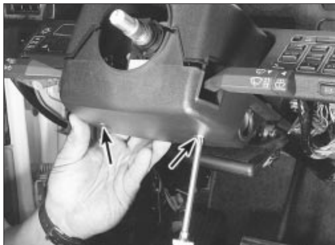
27.3 Remove the lower steering column cover screws
