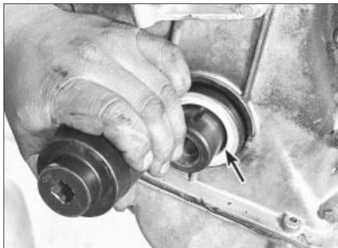
7.11 Drive the new seal squarely into the front cover with a large socket or section of pipe - do not remove the plastic refitting guide (arrowed) until the seal is installed
