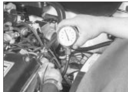
2.4b The oil pressure can be checked by removing the sender unit and refitting a pressure gauge in its place
