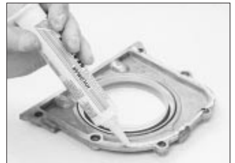
15.5 Apply RTV sealant to the sealing surface
