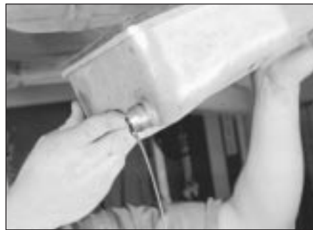
26.8 Lower the sump pan from the transmission
