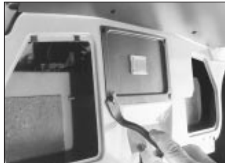
17.6 Detach the clips securing the boot lamp finish panel
