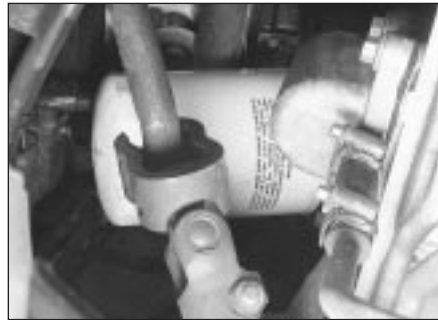
3.13 The oil filter is located on the left side of the engine - use a filter wrench for removal (tighten the new filter by hand)
