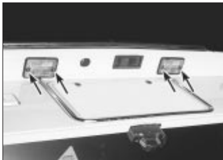
21.6 Detach the lens retaining screws (arrowed) and the lens to access the number plate light bulbs
