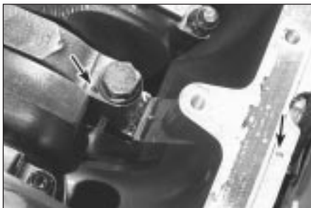
14.5 The right side of each main bearing cap is stamped with a number (left arrow) that corresponds to the stamped number on the pan rail (right arrow)
