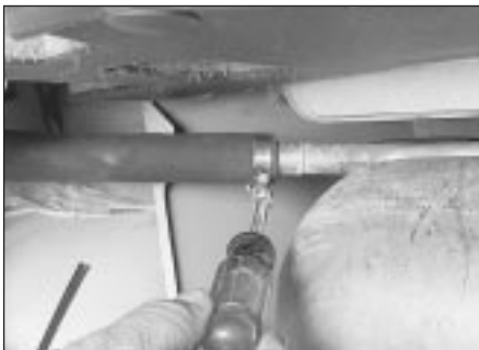
7.9b Disconnect the vapour return line from the fuel tank
