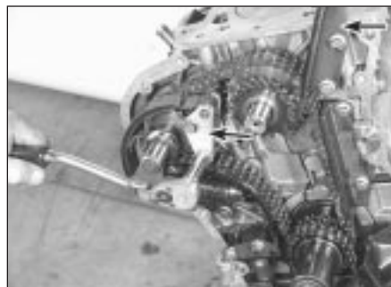
8.12 Unbolt and remove the upper chain guide (right arrow) and the upper chain tensioner guide (left arrow)
