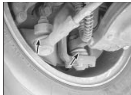
12.10 Inspect the balljoint and tie-rod end boots for tears - tears or damage in either boot will allow contamination of the grease which will lead to premature failure
