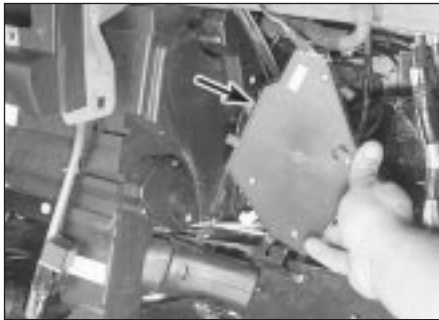
11.6b Pull away the climate control computer (arrowed)
