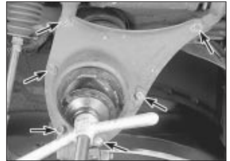
8.3 To detach the coil spring pan from the lower control arm, compress the spring and remove these six bolts (arrowed)
