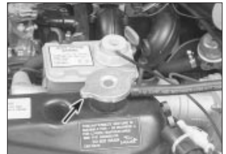
30.3 Push the expansion tank pressure cap downward and rotate anti-clockwise - never remove it when the engine is hot!
