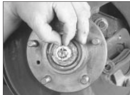
22.23 Position the nut lock on the spindle nut so that it lines up with the cotter pin hole - DO NOT loosen the spindle nut from its snug position
