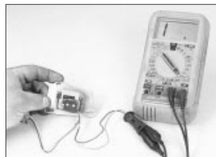
13.7a To check the brake light switch, connect an ohmmeter to the switch terminals; with the switch plunger released, there should be no continuity (infinite resistance)
