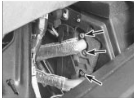
11.5 With the cover off, remove the Allen bolts (arrows indicate three of the four) to pull the coolant pipes out of the left side of the heater core
