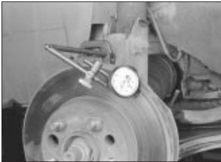
5.4a To check disc runout, mount a dial indicator as shown and rotate the disc
