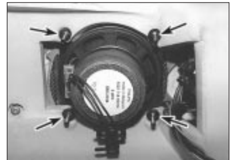
13.6 Remove the nuts from the retaining studs (arrowed) to remove the speaker
