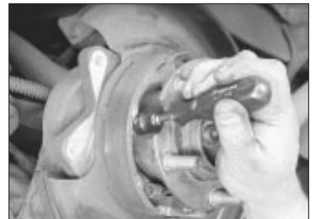
12.5c Remove the front hold-down spring, washers and pin; note that one washer goes below the spring and one above it
