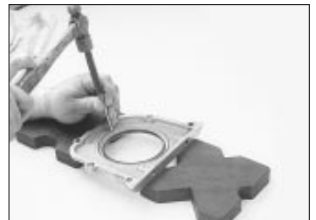
15.3 After removing the retainer assembly from the engine block, support it between two wood blocks and drive out the old seal with a drift punch and hammer
