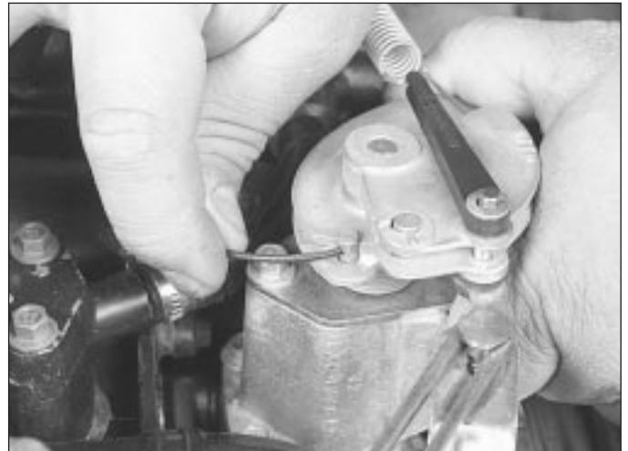
10.3 Rotate the bellcrank and remove the cable end from the slot
