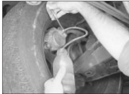
9.9 When bleeding the brakes, a hose is connected to the bleed screw at the caliper or wheel cylinder and then submerged in brake fluid - air will be seen as bubbles in the tube and container (all air must be expelled before moving to the next brake)
