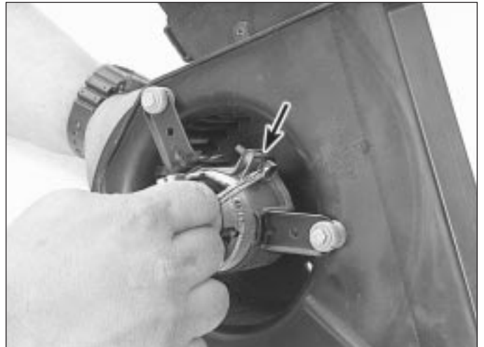
10.11b Loosen the clamp bolt (arrowed) on the motor bracket and then pull the motor and fan out as an assembly
