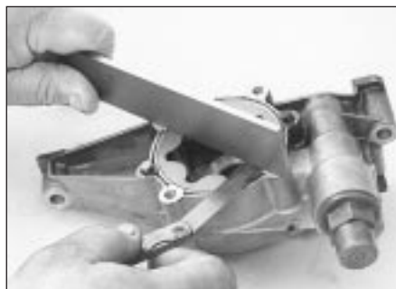
13.10 With a straightedge held tight to the pump surface, measure the clearance over the rotors with feeler gauges
