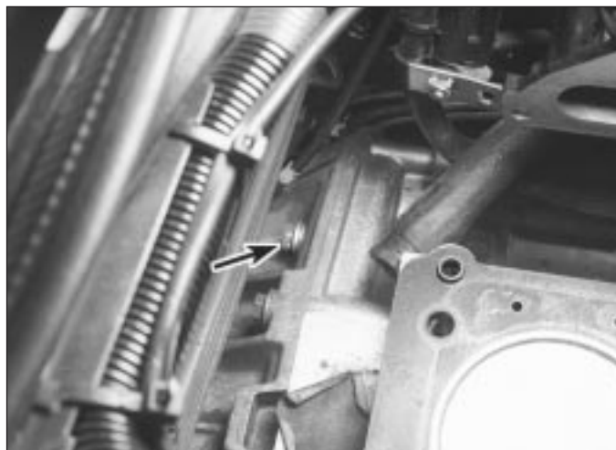
15.5 The upper starter bolt can be reached from underneath the vehicle using a long extension and swivel socket (cylinder head removed for clarity)
