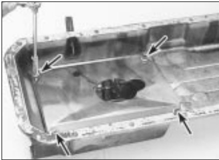
12.8 Remove the bolts (arrowed) and the sheetmetal baffle plate - clean the sump area of the sump with the baffle removed
