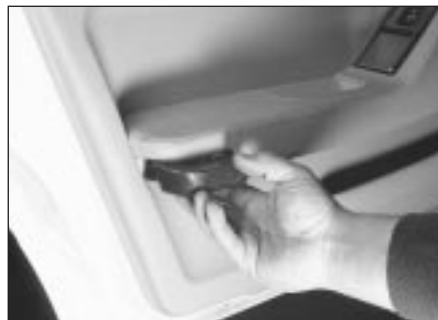
18.7a Prise out the courtesy lamp lens
