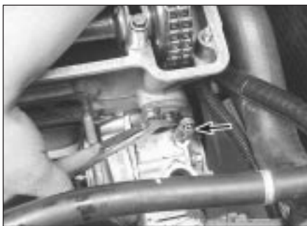
10.7 Loosen this bolt (arrowed) and swing the clamp away from the tensioner, then use pliers to pull the valve out
