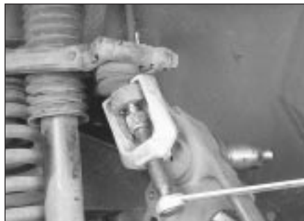
5.7 To detach the upper balljoint from the steering knuckle, loosen the ballstud nut, fit a small puller and break the ballstud loose from the knuckle
