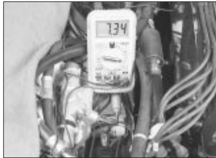
8.3b To check the secondary resistance of the coil, measure the resistance between the positive terminal and the HT terminal
