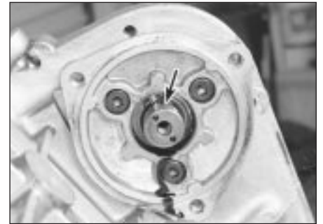
9.5 Use snap-ring pliers to remove the snap ring (arrowed) from the shaft - note the three internal hex-head bolts retaining the housing to the engine block
