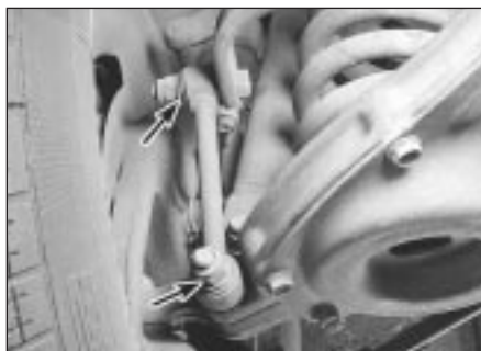
12.8b Check the anti-roll bar bushings (arrowed) for deterioration at the front and the rear of the vehicle
