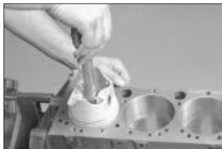
22.3 When checking piston ring end gap, the ring must be square in the cylinder bore (this is done by pushing the ring down with the top of a piston as shown)
