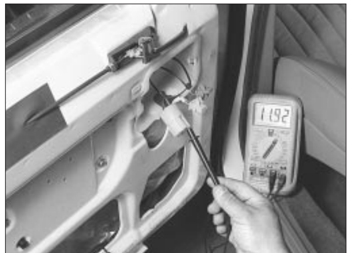
24.12 If no voltage is present at the motor with the switch depressed, check for voltage at the switch
