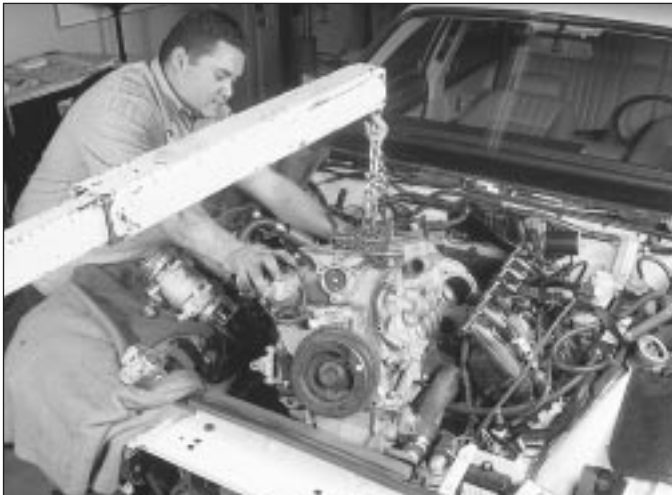
6.20 Lift the engine high enough to clear the vehicle, tilting it up at the front to clear the front crossmember, then move it away and lower the hoist
