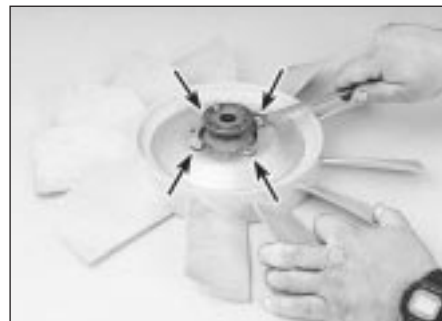
4.12 Separate the fan clutch from the fan by removing the four bolts (arrowed)
