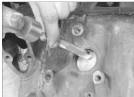
15.1a A hammer and a large punch can be used to knock the core plugs sideways in their bores
