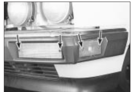
21.1 The front direction indicator/rear parking and side marker light bulbs are accessible after removing the lens screws
