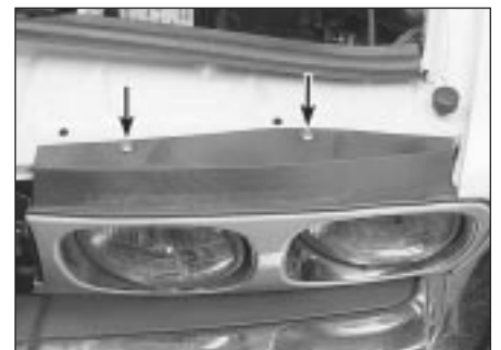
17.2 Remove the screws (arrowed) and detach the headlight bezel trim cover
