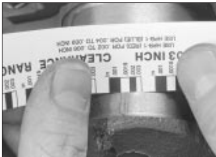
25.17 Measure the width of the crushed Plastigauge to determine the big-end bearing oil clearance
