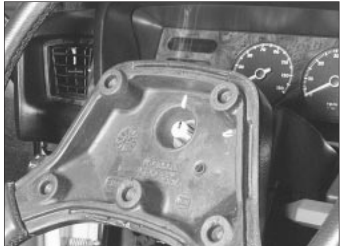
14.3 After removing the steering wheel nut, make a pair of alignment marks on the steering wheel and steering shaft to ensure proper reassembly
