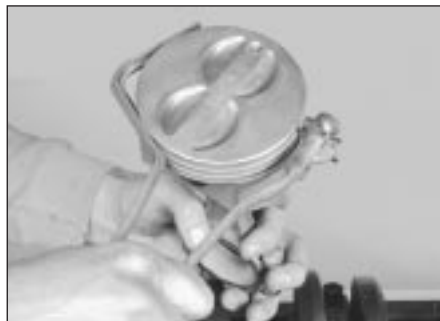
18.4a The piston ring grooves can be cleaned with a special tool, as shown . . .
