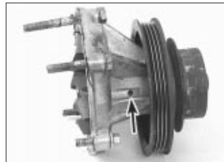
7.3 Check the weep hole (arrowed) for signs of leakage (pump removed for clarity) - grey discoloration is normal, large brown stains indicates seal failure
