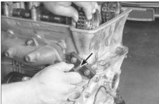
10.28 The special tensioning tool simulates the operation of the oil-driven tensioner - apply 4 to 6 Nm (36 to 48 inch-pounds) pressure on the centre bolt (arrowed)
