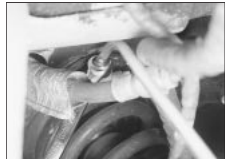
10.2b After depressurising the system, attach a bleed hose to the bleed screw on the left valve block, open the bleed and drain any residual fluid into a catch bottle
