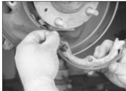
12.5m . . . hook the other end of the lower spring into the rear shoe . . .
