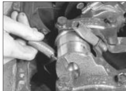
13.6 To prevent damage to the crankshaft journals and cylinder walls, slip sections of hose over the connecting rod bolts before removing the pistons
