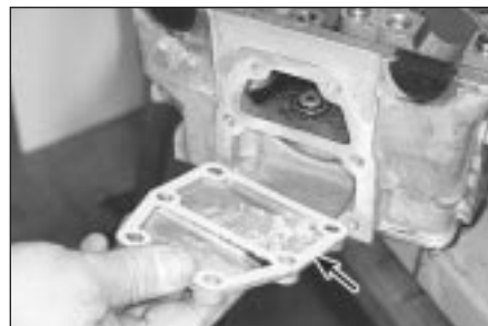
11.19 Remove the rear cover from the cylinder head, clean the gasket surfaces and refit the cover with a new gasket (arrowed) - note that the printed-on sealer bead is placed against the cylinder head
