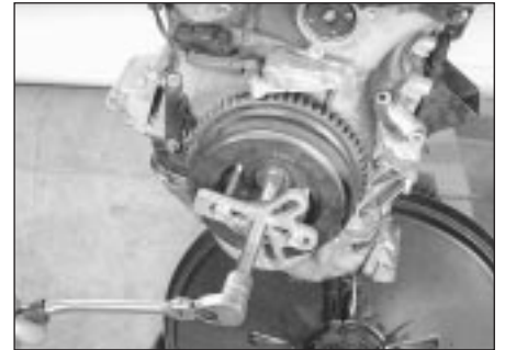
7.5 After removing the centre bolt, remove the crankshaft damper with a two-bolt puller - be careful not to damage the sensor ring
