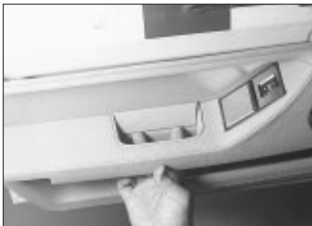
18.8a Push up on the bottom to detach the armrest/pull handle trim cover
