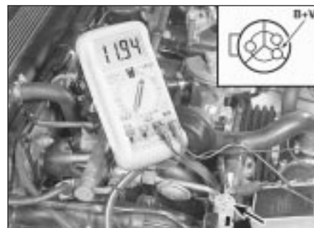
13.49 Check for battery voltage to the supplementary air valve
