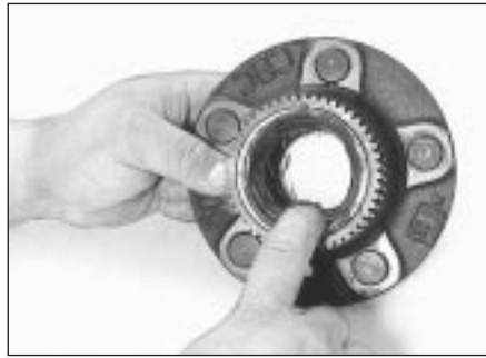
22.17 Apply a thin layer of grease to the inner and outer bearing races
