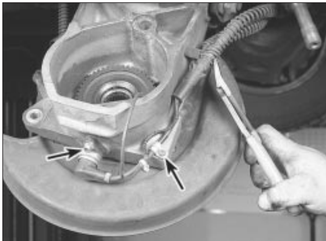
11.4 Before detaching the hub carrier from the rear control arm, remove the ABS sensor (left arrow), detach the ABS harness clip (right arrow) and cut the cable tie securing the harness
