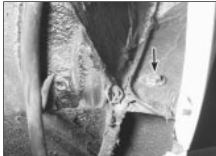
15.7c Working in the wheel opening, remove the wing-to-rocker panel bolt (arrowed)
