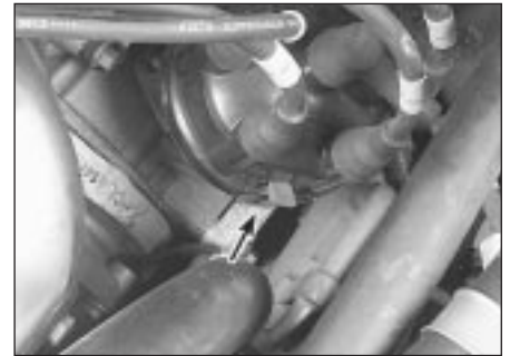
19.11a Unsnap the distributor cap retaining clips - pull the cap up and away to access the rotor
