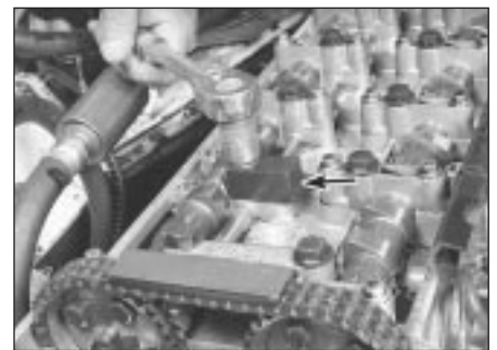
10.10b . . . replace it with the special spacer block (arrowed) and tighten the cylinder head bolt to 53 Nm (39 lbf ft)
