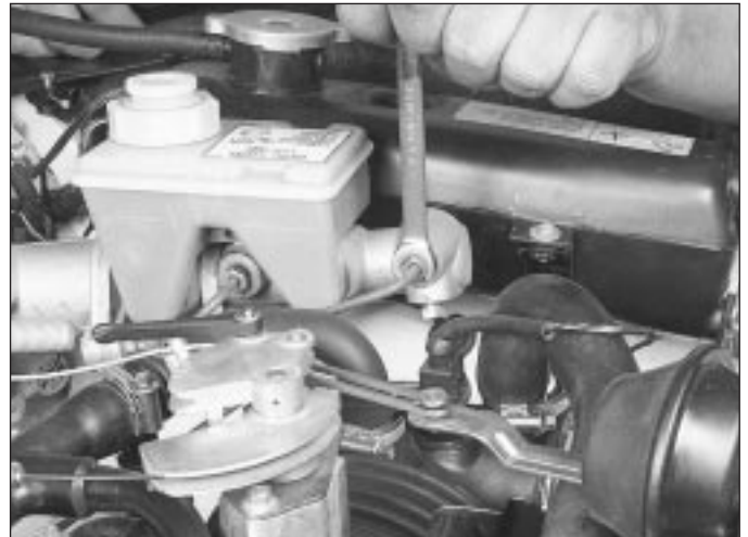
6.5 Loosen the hydraulic brake line fittings with a flare-nut spanner to protect the corners of the nuts
