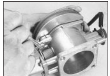
13.20 Adjust the butterfly angle by loosening the locknut on the throttle stop and turning the adjustment bolt
