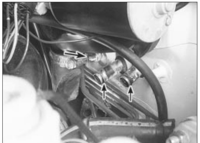
11.2 Disconnect the heater hoses from the pipes at the bulkhead (small arrows) - the large arrow indicates the evaporator case retaining nut
