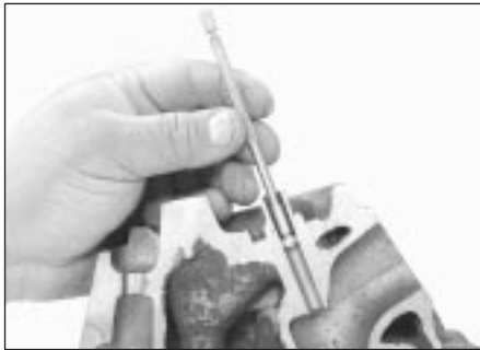
10.15 Use a small dial bore gauge to determine the inside diameter of the valve guides - subtract the valve stem diameter to determine the stem-to-guide clearance
