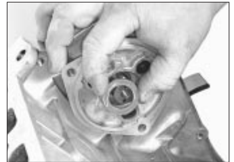
9.10 Refit the washer before replacing the snap-ring
