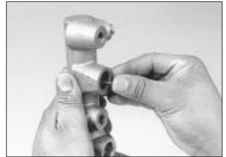
6.7o Using the same technique as in illustration 6.7f, depress the pistons and refit the stopper pin
