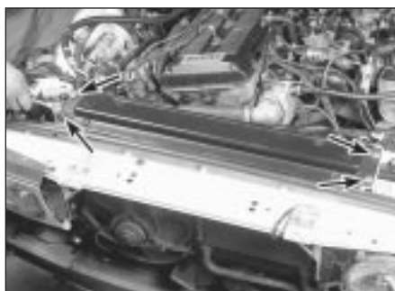
5.6 Remove the bolts (arrowed) and take off the radiator cowl panel
