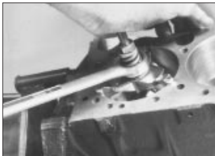
13.1 A ridge reamer is required to remove the ridge from the top of each cylinder - do this before removing the pistons!
