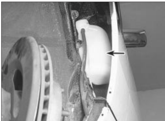
5.17 The recovery bottle (arrowed) on 1988 and 1989 models is located in the footwell - disconnect the hoses and the two mounting screws
