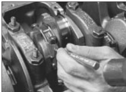
13.4 The connecting rods and caps should be marked by cylinder number - if they aren't, mark them with a centre punch to avoid confusion during reassembly
