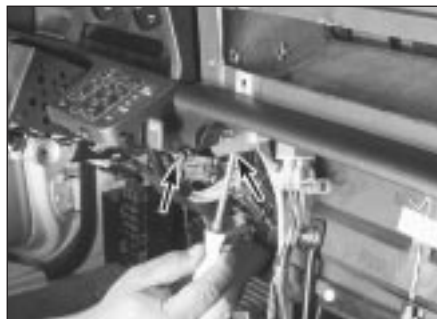
25.4 Working in the knee bolster opening, remove two retaining screws from each end of the instrument cluster housing
