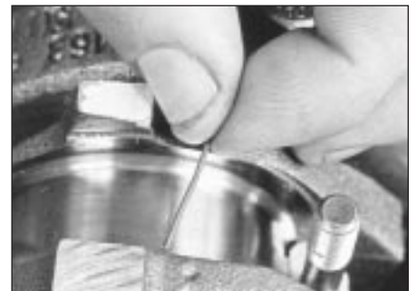
25.13 Lay the Plastigauge strips on each big-end bearing journal, parallel to the crankshaft centreline
