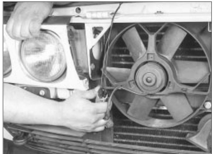
4.17 Disconnect the fan wiring connector and connect jumper wires from there directly to the positive and negative terminals of the battery - the purple wire's terminal should receive the battery power and the black wire's terminal should be earthed
