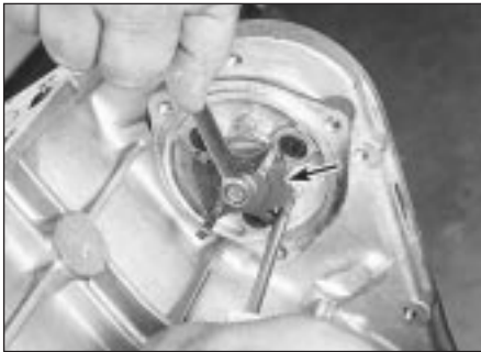
9.3 Use a screwdriver to hold the drive coupling (arrowed) stationary while removing the bolt
