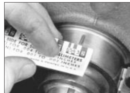
23.14 Compare the width of the crushed Plastigauge to the scale on the envelope to determine the main bearing oil clearance (always take the measurement at the widest point of the Plastigauge). Be sure to use the correct scale - imperial and metric scales are included
