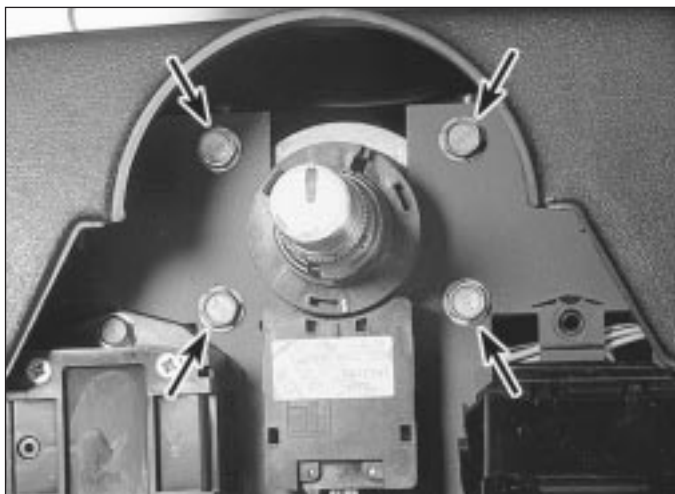
9.4 Remove the switch mounting plate screws (arrowed). Lower the mounting plate and switch assembly to access the ignition switch/key lock cylinder
