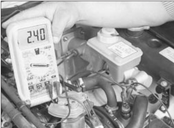
4.51 The air intake temperature sensor resistance will DECREASE when the temperature of the air INCREASES
