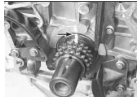
8.16 Apply paint marks on the crankshaft, crankshaft sprocket and the engine block (arrowed) to indicate TDC position
