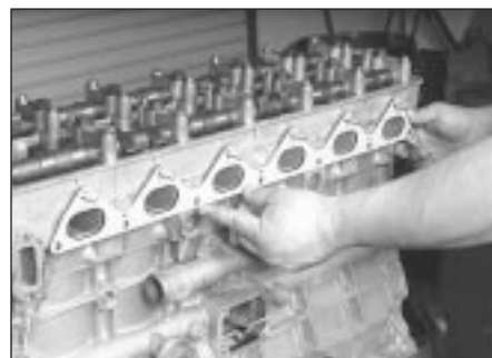
5.9 Refit the new intake manifold gasket over the studs (arrowed) refit the manifold
