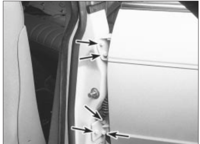
19.7b Open the front door to access the rear door hinge-to-body bolts (arrowed)
