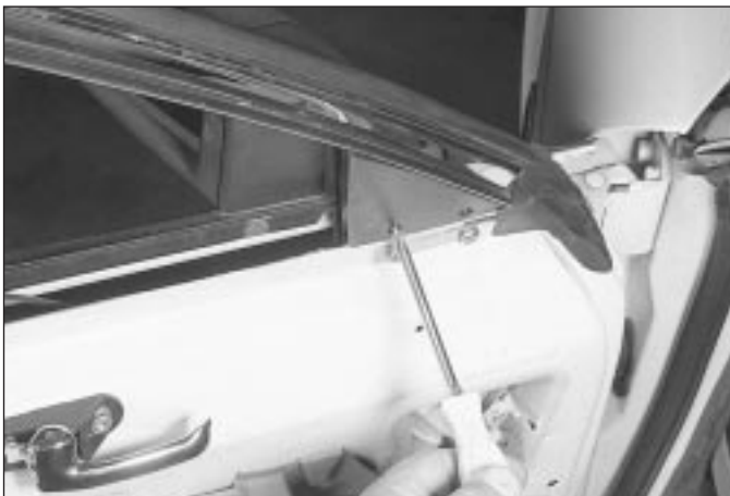
23.2 Remove the trim cover retaining screws
