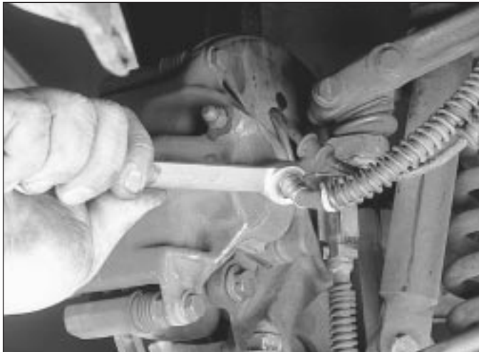
4.2 Use a flare-nut spanner to protect the brake hose fitting when unscrewing it from the caliper
