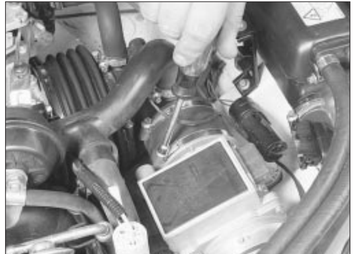
13.8 Remove the air intake duct clamp from the MAF sensor housing
