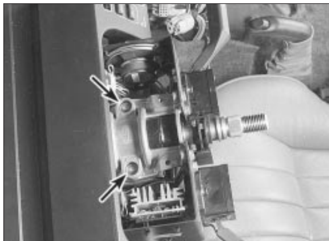
9.5 To remove the ignition switch/lock cylinder assembly, drill out the centre of the two retaining bolts (arrowed) and remove them with a screw extractor
