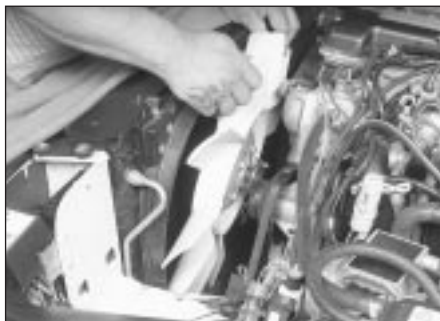
4.9 The fan can be removed with the shroud in place by angling it out of the shroud
