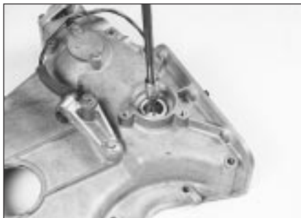
8.28a Drill a small hole in the intermediate shaft seal, thread a sheet metal screw into it and use a small slide-hammer pull the seal out of the cover
