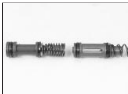
6.7k Refit the new O-ring seals and cups as shown; make sure the cups on the primary piston (the one on the left) face forward as shown (toward the spring), and the cups on the secondary piston (the one on the right) face out, away from the piston (the one on the left faces toward the primary piston, the one on the right faces toward the spring)
