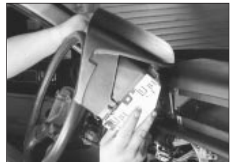
25.5 Pull outward on the instrument cluster housing and unplug the electrical connectors from the backside
