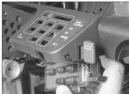
10.2 Depress the clip on the front, lower the switch assembly from the instrument panel and unplug the connectors
