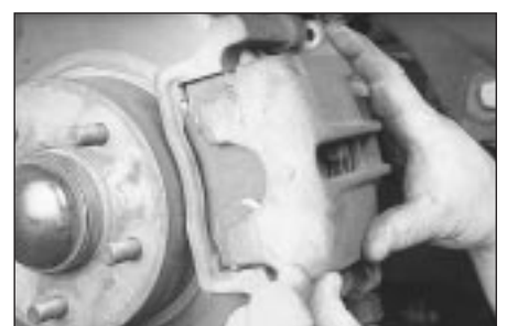
3.5o Refit the caliper, then tighten the mounting bolts to the specified torque
