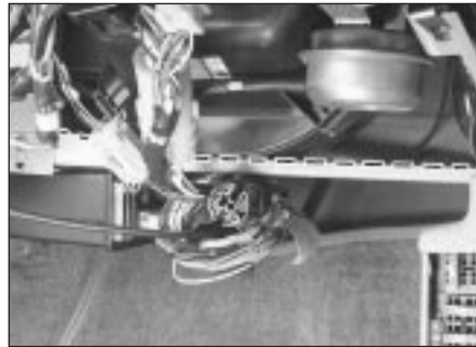
10.2b Apply heavy duct tape to the sharp edge of this brace (dotted line) when working behind the glove box area of the dash - the metal is very sharp
