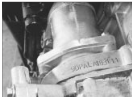
The engine identification number is stamped on the right side of the engine block just behind the distributor
