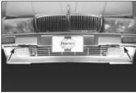
14.3 Remove the two retaining bolts from the bottom of the bumper, then remove the bumper from the vehicle
