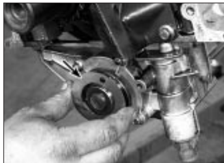
13.17 Refit the original shim pack (arrowed) if the original pump is being used - if a new pump is being installed, refit a 0.38 mm (0.015-inch) shim pack
