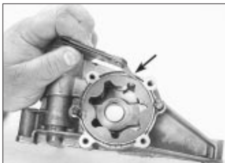
13.9 Measure the outer rotor-to-body clearance with feeler gauges (arrowed)
