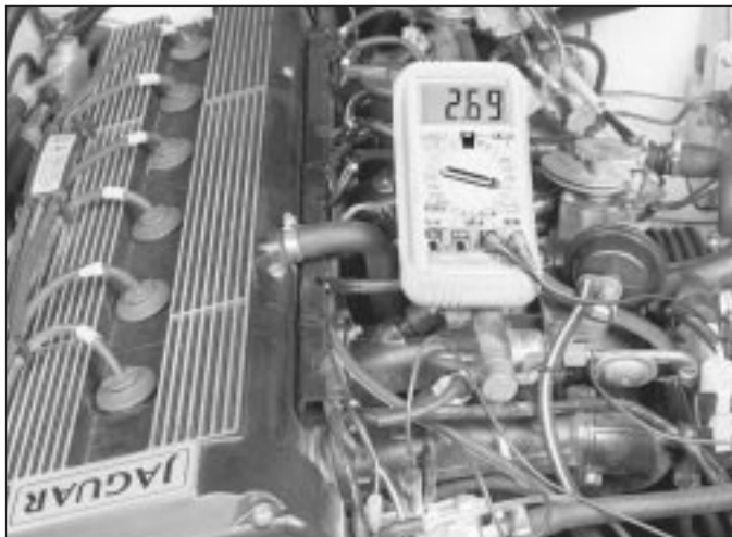
4.2 The coolant temperature sensor is in the thermostat housing. To check the coolant temperature sensor, use an ohmmeter to measure the resistance between the two sensor terminals
