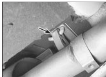
14.1b Check the condition of the flexible rubber mounts that hang the silencer to the chassis
