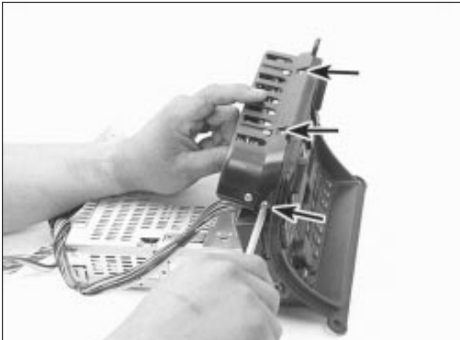
12.3b Remove the four screws (three are shown here) holding the control assembly in the control/radio housing
