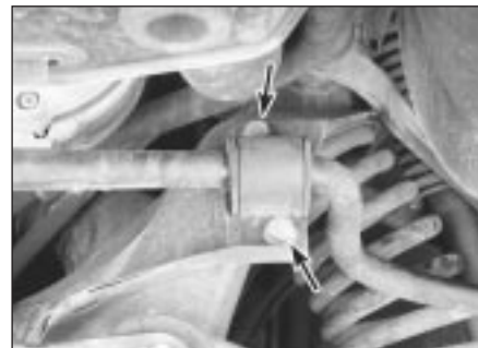
3.2 To detach the anti-roll bar from the suspension crossmember, remove these two bolts (arrowed) from each bushing bracket
