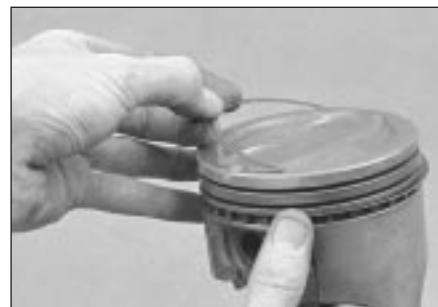
22.9b DO NOT use a piston ring refitting tool when refitting the oil ring side rails
