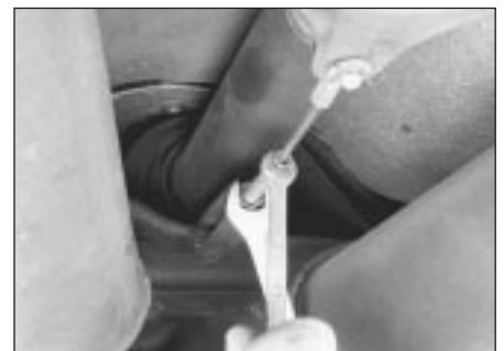
10.3 To adjust the handbrake cable, loosen the locknut, then turn the adjuster to remove any slack in the cable; be sure to tighten the locknut when the cable is properly adjusted
