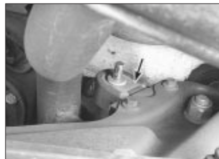
10.2 Check the exhaust system hangers (arrowed) for damage and cracks
