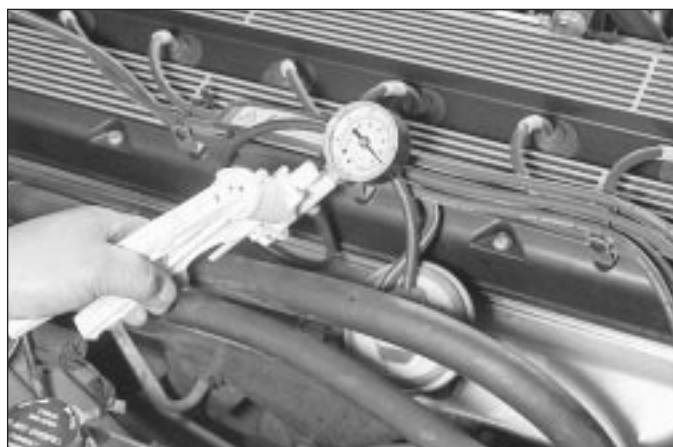
6.4 Apply vacuum to the EGR valve and confirm that the valve opens and allows exhaust gases to circulate. Once it is activated, the EGR valve should hold steady (no loss in vacuum)
