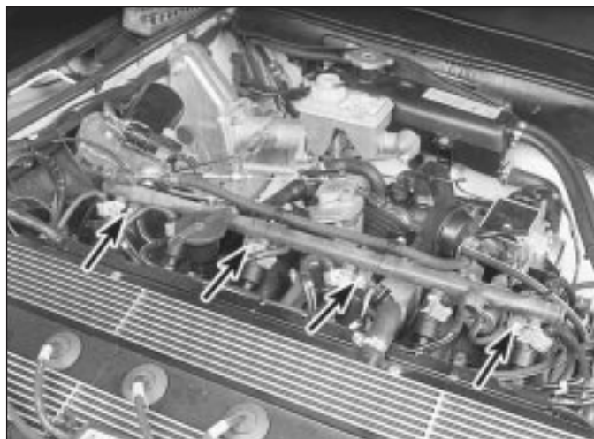
13.35 Remove the fuel rail mounting bolts (arrowed) . . .
