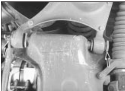
9.4 To detach the lower control arm from the crossmember, remove this nut and bolt (arrowed) (unbolt and lower the steering gear before you can pull out the pivot bolt)
