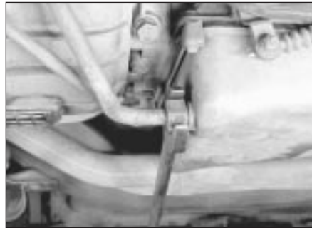
26.6a Unscrew the dipstick tube collar
