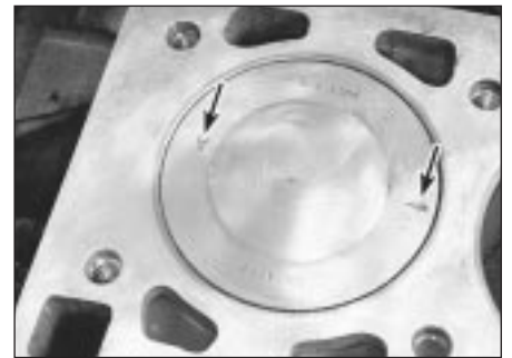
25.9 Pistons must be installed with the arrow (right arrow) or FRONT facing the front of the engine - left arrow indicates piston size letter
