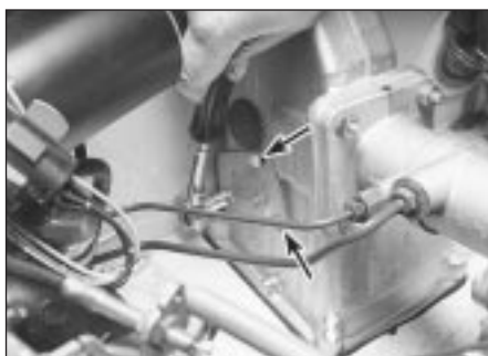
13.6a To remove the brake light switch, remove the three mounting plate screws (arrowed) . . .
