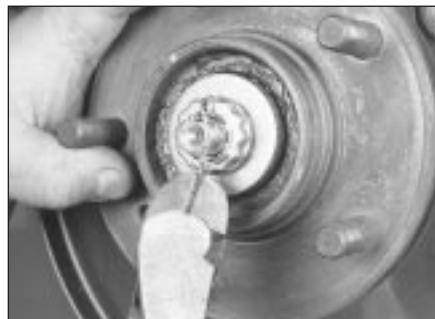
22.7 Remove the cotter pin and discard it - use a new one when the hub is reinstalled
