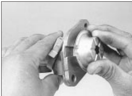
6.7p Refit the end plate as shown, with the bend in the plate flange aligned with the groove in the master cylinder flange
