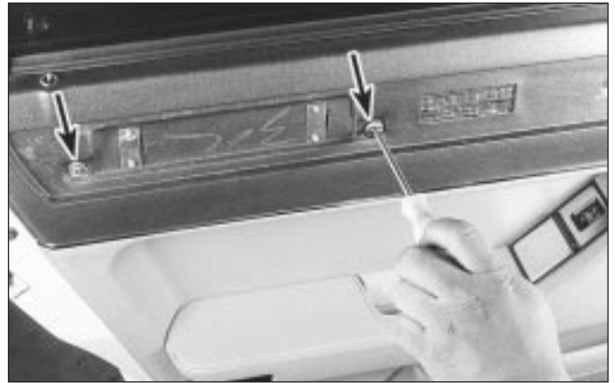
18.5 Detach the screws located behind the wood finisher panel, then remove the upper portion of the door trim panel
