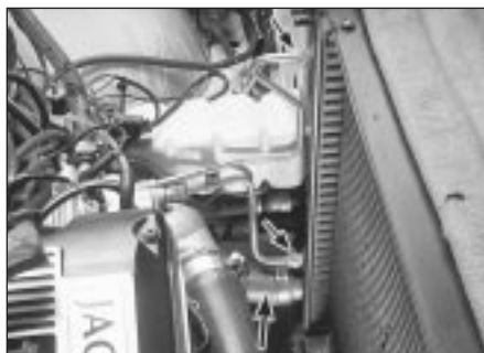
5.5a At the left side of the radiator, disconnect the automatic transmission cooler lines (small arrows) and the lower radiator hose (larger arrow)
