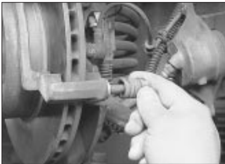
3.5i Remove the caliper guide pins and boots (lower pin and boot shown) . . .
