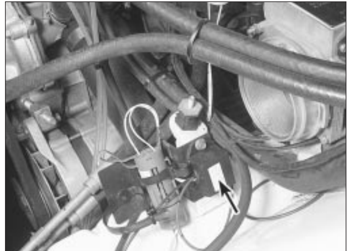
11.9 The load dump module is located on the bulkhead next to the MAF sensor
