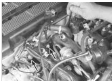
5.7b Remove the intake manifold bolts/nuts and remove the intake manifold - the upper fasteners are studs/nuts, while the lower row are bolts (two arrowed)
