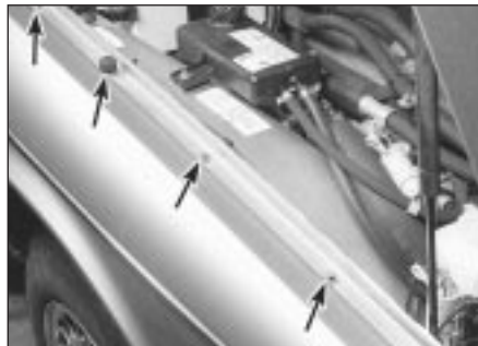
15.7e Detach the bolts along the top of the wing
