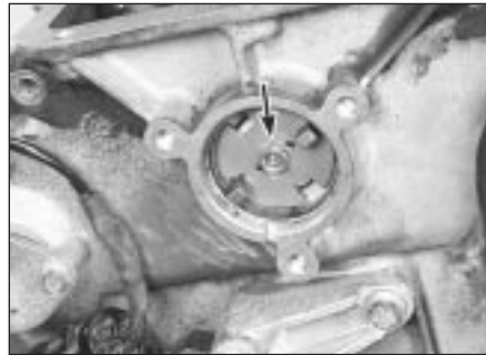
8.9b . . . and unbolt the drive coupling (arrowed) from the intermediate shaft
