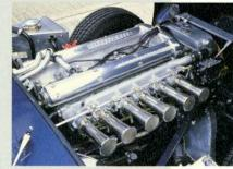
sump lubrication. Even alloy cylinder blocks are available if desired. With a power output of up to 340 bhp, its performance is stunning with 0-60mph in 4.4 seconds and 0-100mph in 10.9 seconds.
