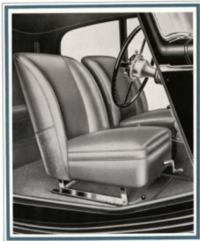
Both front seats are adjustable, not only for fore and aft movement but for height and pitch. When the most suitable position for each has been secured by use of the lateral slides, the seat can be raised or lowered until the ideal individual driving position is attained. Both adjustments are finger tight and can be carried out whilst the driver remains seated (fitted to 3½ and 2½ Litre closed models and "Special Equipment" 1½ Litre model).
