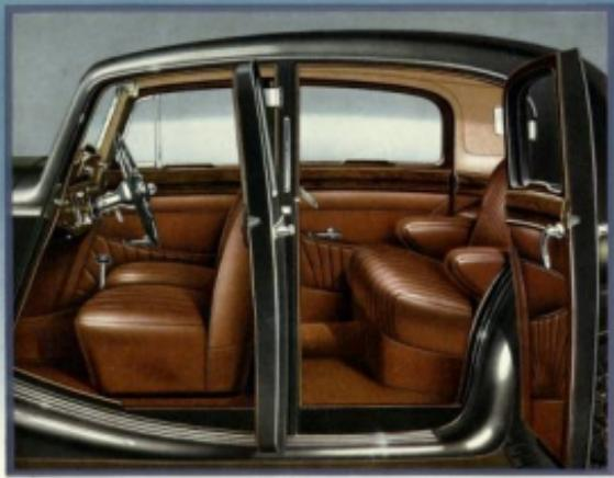
The luxuriously appointed interior affords full accommodation for five persons. Wide doors and flat floor make ingress and egress particularly easy. Draughtless ventilating half windows are fitted to front doors, whilst the sliding roof is of flush fitting single action type. Large pockets are provided in all doors.
