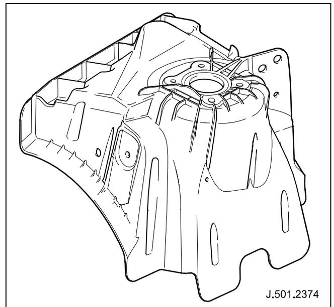
Fig. 137 Typical casting (448 alloy)
