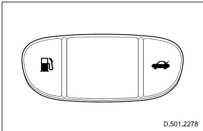
**Fig. 155 Fuel filler-flap/luggage compartment lid release**
