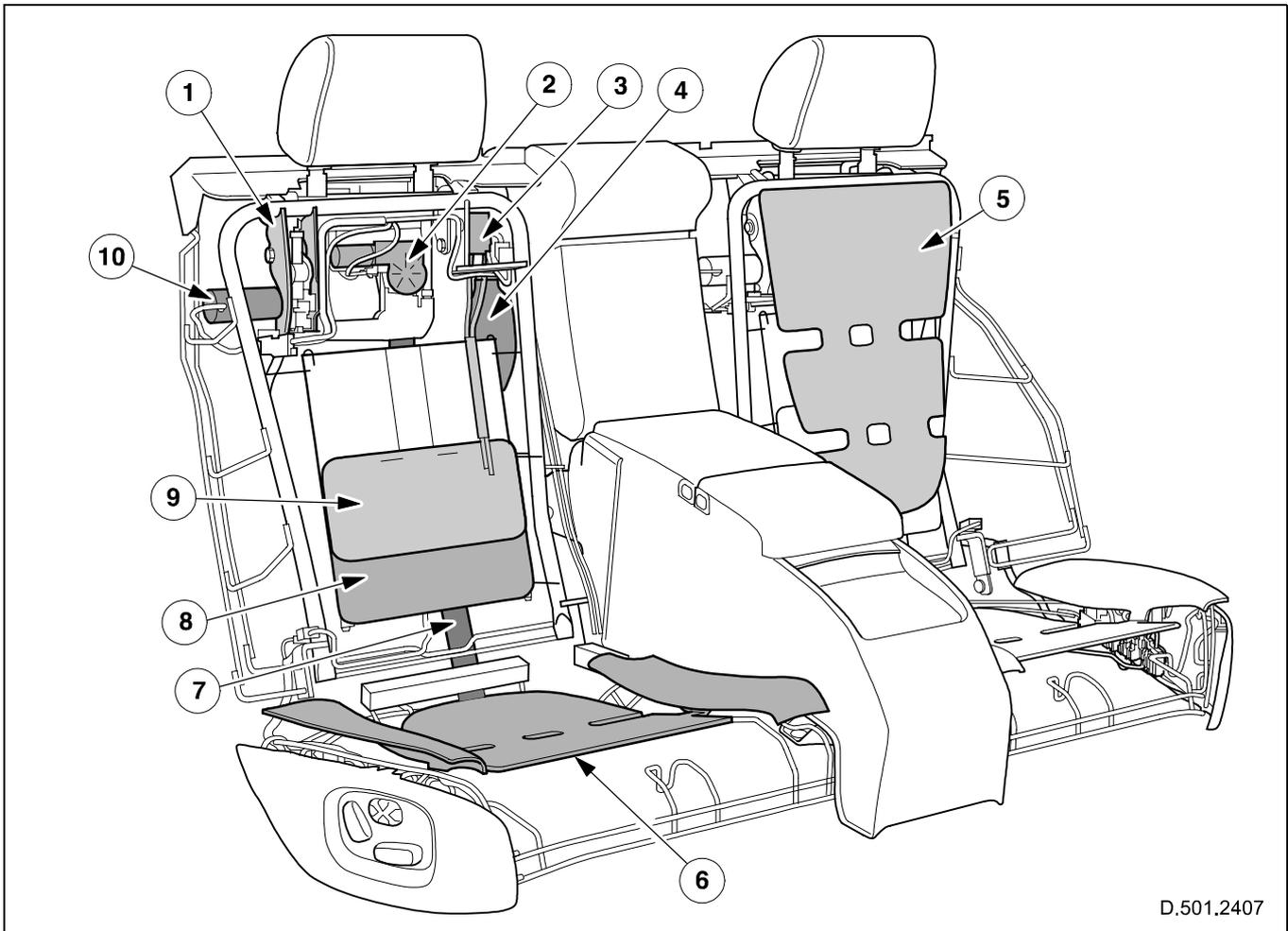
**Fig. 147 Electrically-adjustable twin rear seats**
