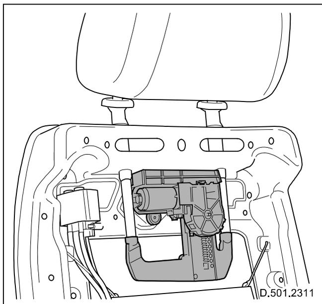
Fig. 143 Electrically operated head restraint
