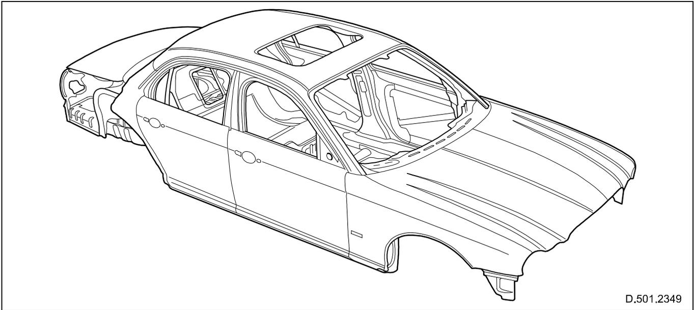
Fig. 136 Body shell with closures
