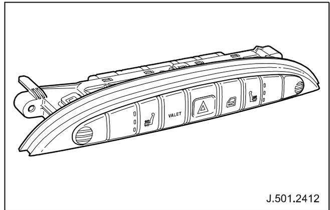
**Fig. 156 Center console switch assembly**
