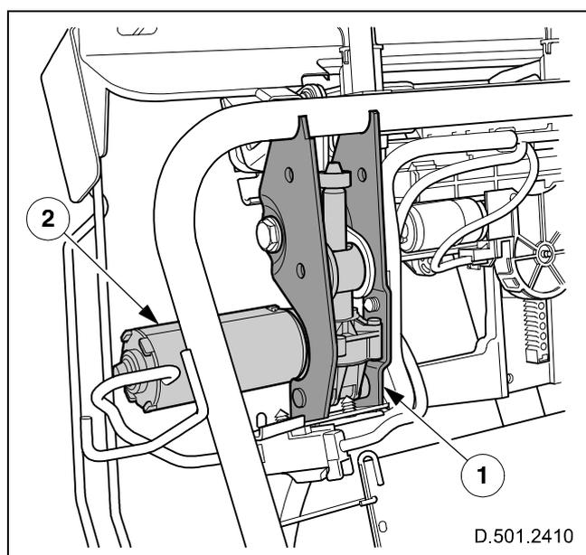
**Fig. 146** Electrically-adjustable backrest
