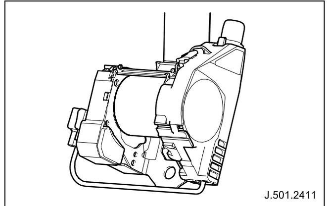
Fig. 174 Retractor-type pre-tensioner (rear center)
