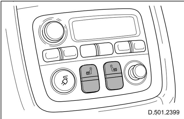
**Fig. 152 Heated seat switches (4-zone console)**
