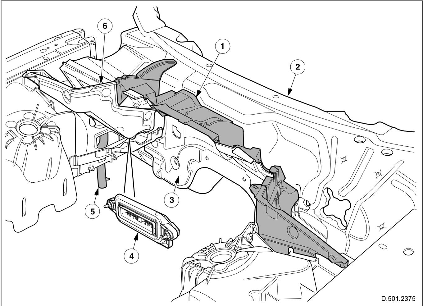
**Fig. 139 Secondary bulkhead location**
