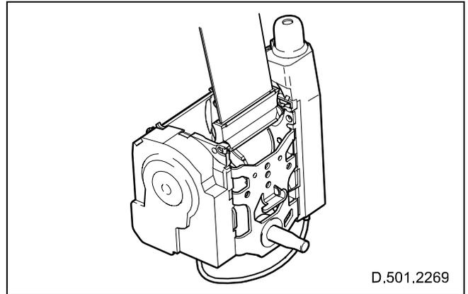
Fig. 175 Retractor-type pre-tensioner (rear left-hand)
