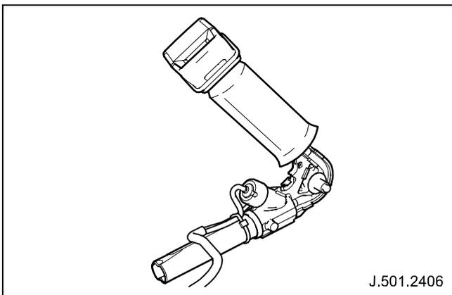
Fig. 173 Buckle-type pre-tensioner
