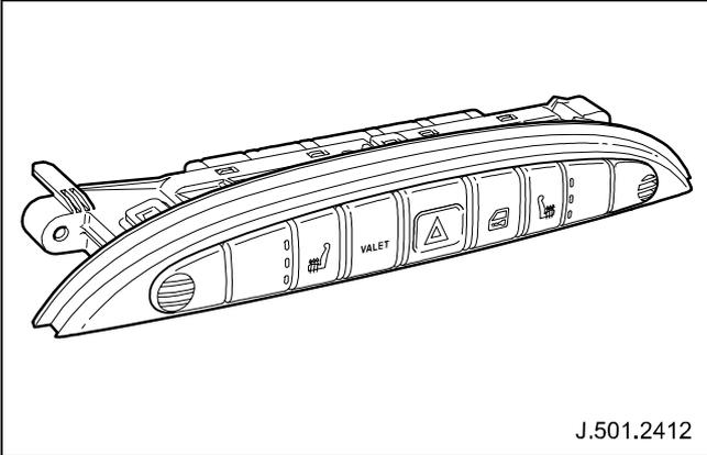
Fig. 145 Heated seat switches
