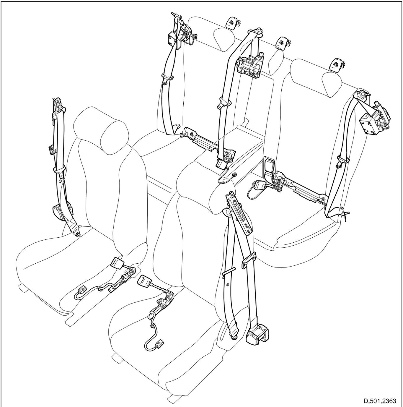
Fig. 164 Occupant restraints - location of active components
