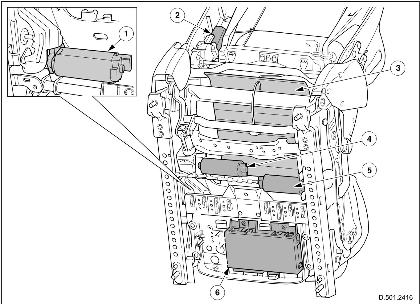
**Fig. 140 Driver power-seat - component locations**
