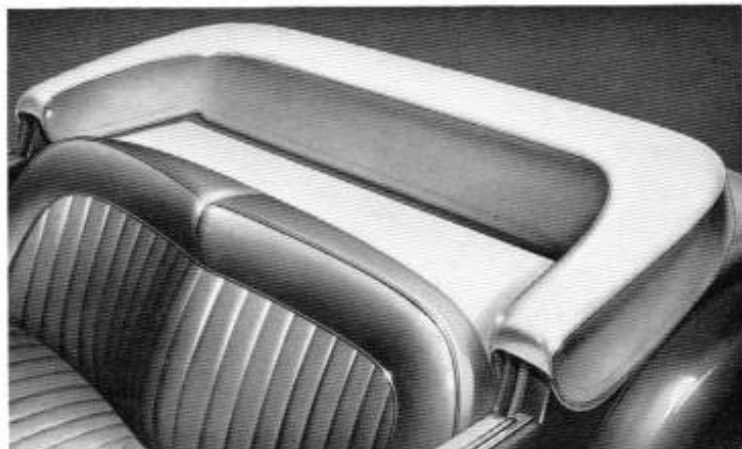
The fully padded and lined hood is easily folded, and when in this position is covered by a neat tonneau which is instantly removable.
