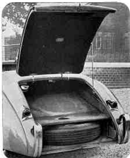
TOURING ESSENTIAL. —The luggage locker is of useful capacity, or can enclose a second spare wheel for competition purposes.
