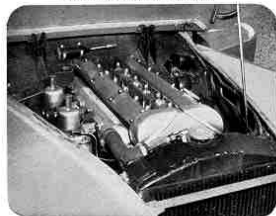
CLASSIC STYLE. —Twin chain-driven overhead camshafts and horizontal S.U. carburetors are features of the neat 6-cylinder, 3½-litre engine.
