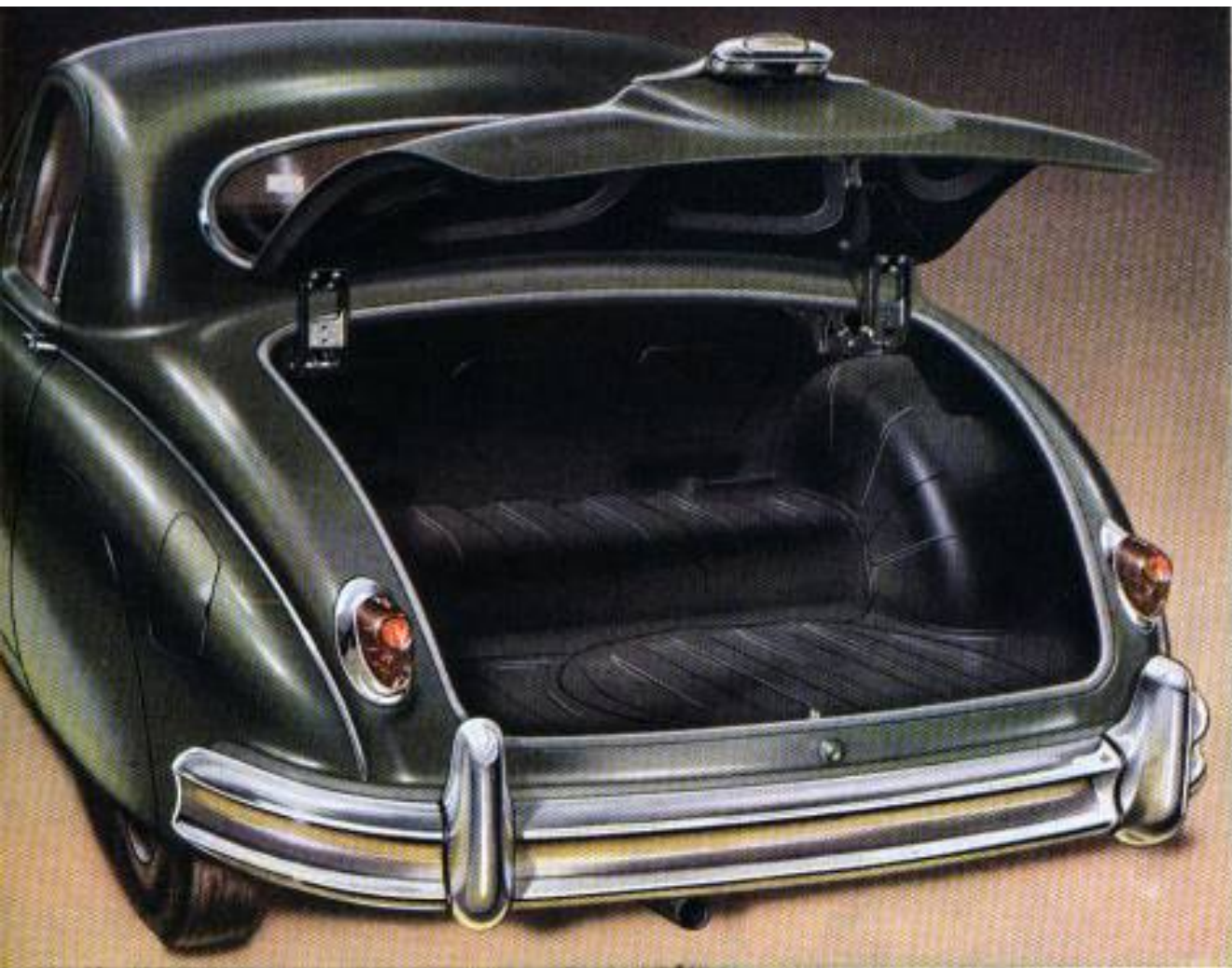
The luggage compartment is of extremely generous dimensions having a capacity of 13.5 cubic feet. An interior light is provided to facilitate the handling of luggage at night.
