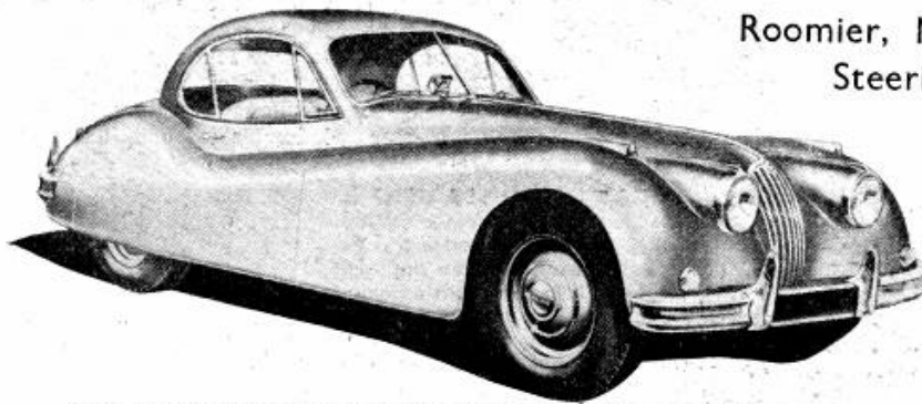
BOLDER grille bars and sturdier bumpers distinguish the XK140 from the 120, this model being the hard-top coupé which has the roof extended rearwards to permit occasional extra seating, and wider doors.
