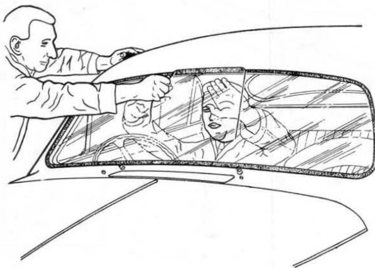
Fig.12.17. Fitting the windscreen to Mk 1 cars
