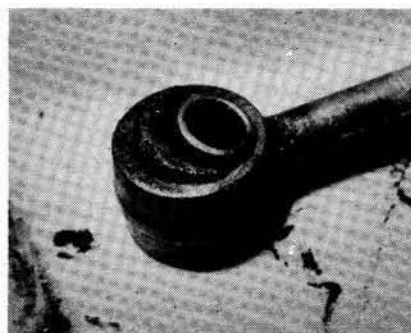
47.1. Engine stabiliser - perished rubber
