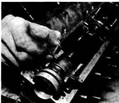
15.2. Camshaft bearing cap 'D' washer
