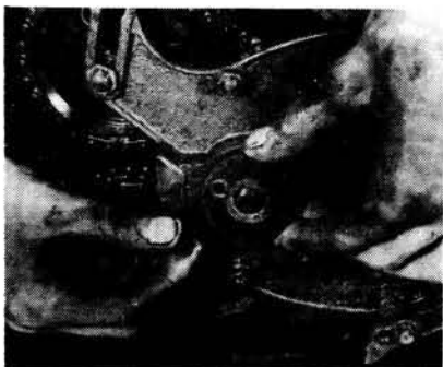
19.4b. Removing serrated plate and spring loaded plunger
