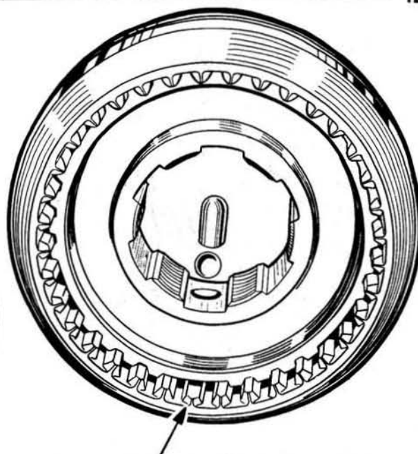
Fig. 6.13. The relieved tooth must be in line with the ball and plunger holes
