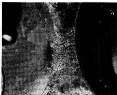
41.2. Burning and cracking of cylinder head
