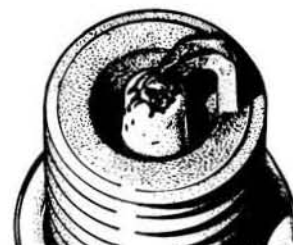
Fig. 4.11. Burning; due to pre-ignition or plug of wrong heat value
