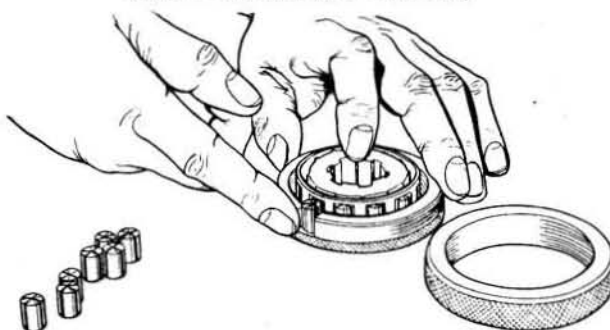
Fig.6.34. Assembly of the uni-directional clutch rollers
