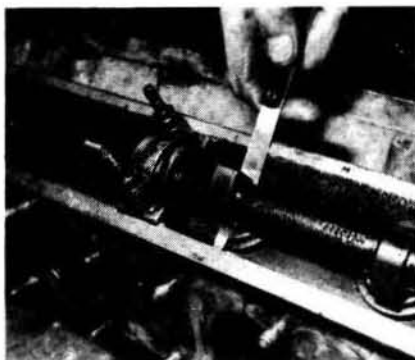
71.5. Checking tappet clearance
