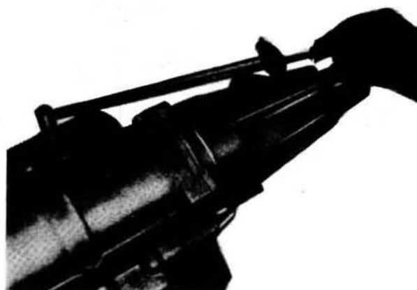
Fig.6.47. Adjusting the rear brake band
