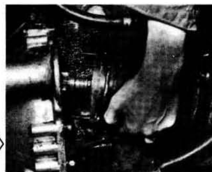
8.1a. Remove starter securing bolts
