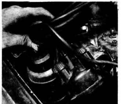
5.40b. Remove distributor head and plug lead harness
