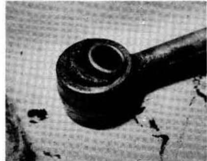
47.1. Engine stabiliser - perished rubber
