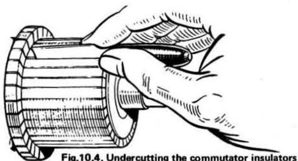
Fig.10.4. Undercutting the commutator insulators
