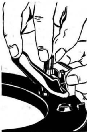
Fig.5.10. Disengaging the strut from the lever
