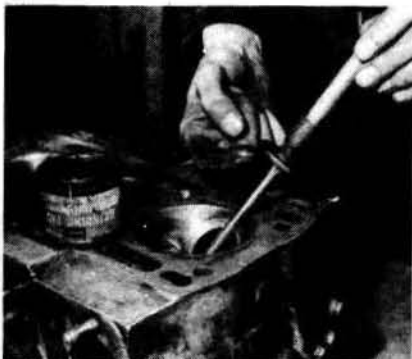
37.5b. Smear of carborundum paste on valve
