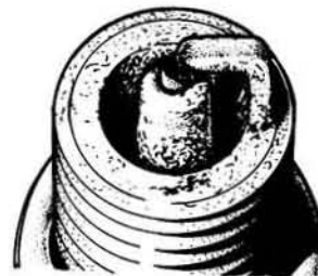
Fig. 4.10. Weak fuel mixture
