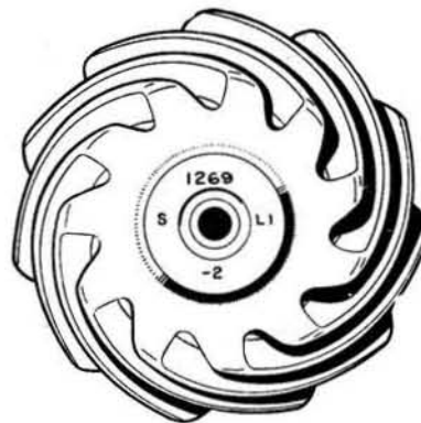
Fig.8.15. Markings on pinion
