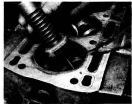
41.4b. Valve seat refacing stone
