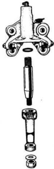
Fig.11.28. Exploded view of the steering idler assembly (early type)
