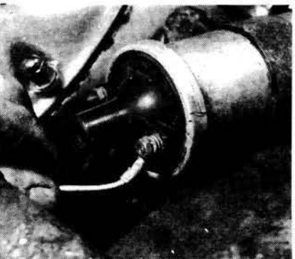
5.41a. Remove leads to coil
