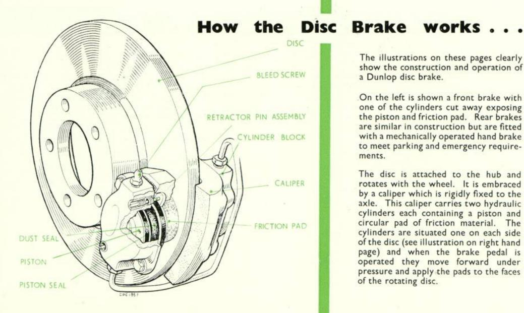
The illustrations on these pages clearly show the construction and operation of a Dunlop disc brake.
