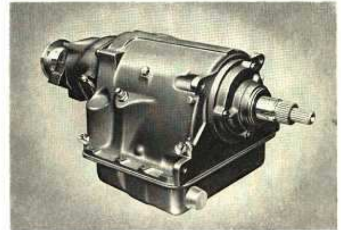
AUTOMATIC TRANSMISSION. Borg Warner Model 8—extensively tested and proven—to match the high torque of the Jaguar 4.2 litre engine. D1/D2 dual drive range gives smooth shifts and option of first or second gear starts as well as full engine braking.
