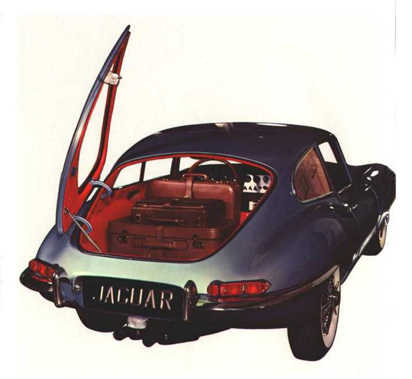
Large counterbalanced door at rear, with release catch located in ear, incorporates window and gives unobstructed access to luggage compartment, spare wheel and tools; hinged luggage container behind seats drops down to increase floor space if desired.
