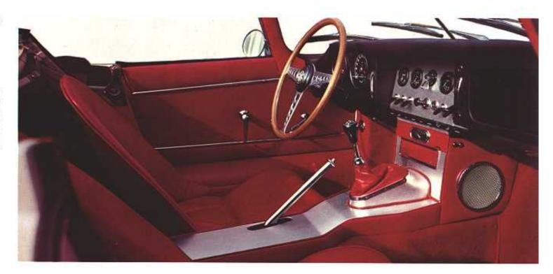
Interchangeable hard or soft convertible top. Three section instrument panel, with r.p.m. counter, 160 m.p.h. speedometer; oil pressure, water temperature and fuel gauges; fuel and brake fluid warning lights.
