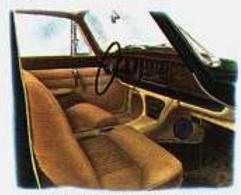
A comprehensive range of instruments, together with a row of switches controlling electrical equipment, are mounted in a polished walnut instrument panel.
