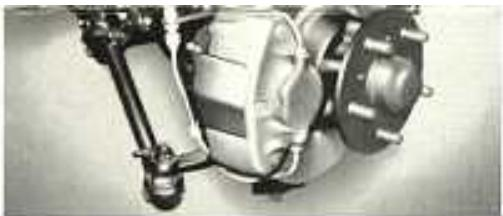
**NEW EFFORTLESS BRAKING.** New brake servo gives lower effort and greater power for the disc brakes on all four wheels. Separate fluid system for front and rear.
