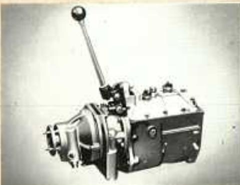
**NEW ALL SYNCHROMESH GEARBOX.** Four speed all synchro, crash proof transmission gives smooth and rapid changes. New diaphragm spring clutch gives lighter pedal pressure and long life. Overdrive available.
