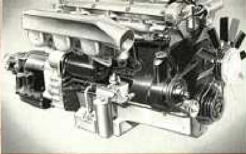
**NEW ADVANCED XK ENGINE.** 4.2 litre, 6 cylinder, twin overhead camshaft advanced design of race-proven, 3 carburettor Jaguar XK engine, five times winner of Le Mans, gives higher torque for increased acceleration and flexibility.
