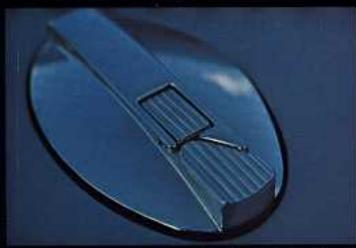
Jaguar XJ6 is equipped with Remote controlled two, not one, gas tanks with side-mounted mirror hinged lockable filler caps. on the driver's side. Each tank holds 12 gallons.
