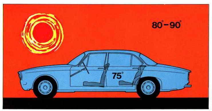
In this condition the automatic air conditioning system would select full cooling to bring temperature down to chosen level of say 75°
