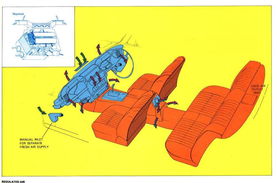
Intermediate temperatures are obtained by varying the mixture of cooled and heated air. In this operational mode the upper flaps
