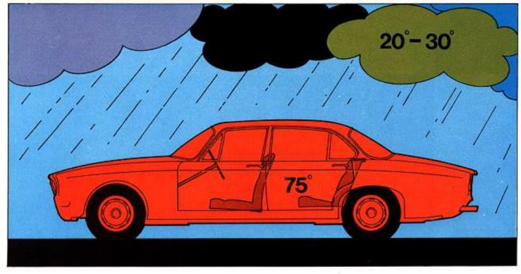
In this condition the automatic air conditioning system would select full heating to bring temperature up to chosen level.
