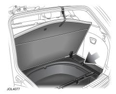
There is an underfloor storage tray located below the floor panel. Lift the floor panel (there is a handle on the rear edge) to access the storage tray.
