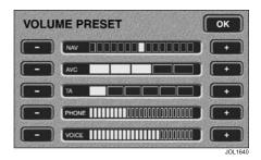
This maintains radio volume at a level sufficient to overcome road noise as vehicle speed increases or decreases.
