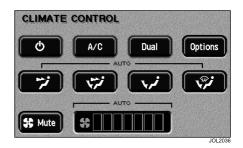
Automatic operation provides a controlled environment over a temperature range of 17°C (61°F) to 31°C (89°F) and should be regarded as the normal operating mode.
