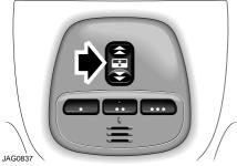
The sunroof switch is located in the overhead console. The ignition switch must be in position **II** for the sunroof to operate.
