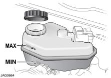
The fluid is visible through the translucent casing of the reservoir and must be maintained at the MAX mark.
