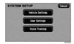
After touching the **System Setup** button, the screen displays the buttons for selecting user settings or vehicle settings.
