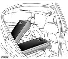
**Wagon:** Release catches are located on the top of each seat back. Press the catch to release the seat back.
