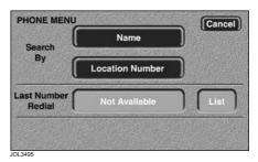
Touch **Menu** to display the above screen. This screen provides access to memory functions and last number redial.
