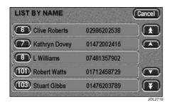
With the memory list displayed above, scroll through the list of names using the arrowed buttons. Touch the desired list number to make the call.
