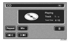
In **CD** mode, touch-screen buttons (shown above) provide selection of CD tracks.
