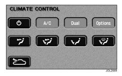
With the climate control system switched off, air recirculation is automatically selected (intake flap closed).
