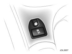
The system will intervene to prevent wheel spin, by automatically reducing the power output from the engine and applying braking to individual wheels.
