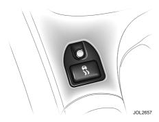
Dynamic stability control (DSC) is operational whenever the engine is running, unless it has been switched off. If the system is operating, the warning light in the instrument panel will flash.
