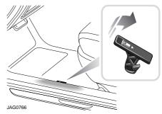
Pull the fuel filler flap release. This is located on the floor, outboard of the driver's seat. See "FUEL TANK FILLING" on page 136.
