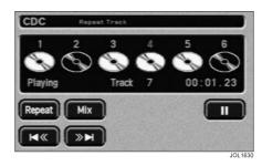
In CD changer mode, touch-screen buttons (shown above) provide for track and disc selection. Discs present in the magazine are highlighted in the display.
