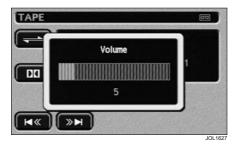
Turn the control knob clockwise to increase or counterclockwise to decrease volume, across a range of settings (0 – 35) to be displayed during and momentarily after adjustment.
