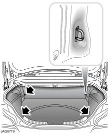
Four metal loops are positioned in the luggage compartment for attaching straps to secure loads and prevent them from sliding over the luggage floor.
