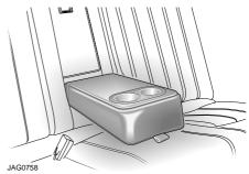
Pull the loop on the rear centre armrest to lower. If not required, raise the armrest to its upright position and push firmly into place. Ensure that the armrest is raised when lowering the seat back to increase the luggage compartment area. See "CUPHOLDERS" on page 120.
