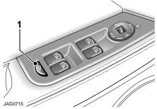
Switches on the driver's door switch pack control the driver and passenger door windows.
