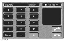
The message window to the right of the screen will provide information on the telephone system's status. If the phone is connected correctly then the display will show **Phone Connected**, or if the phone is not connected to the vehicle, **Discover Me** will be displayed.
