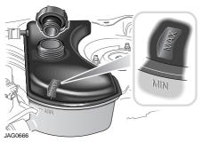
The coolant level must only be checked when the engine is COLD.
