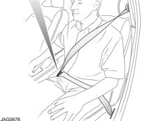
Draw the tongue of the seat belt over the shoulder, across the chest and push it into the buckle unit slot 1. A positive click indicates that it is safely locked.
