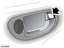
To lock all the doors, press the lock lever on either of the front doors.
