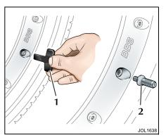
'R' performance wheels – These wheels have a slotted screw valve cover on the wheel face. A pouch containing a 'T'-shaped screwdriver and a valve adaptor, for use with these wheels, is stowed in the glove compartment.
