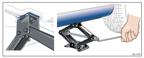
Before raising the vehicle slacken but do not remove the wheel nuts.
