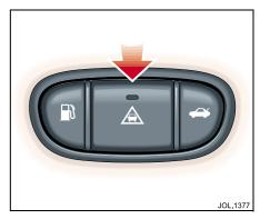
When ACC is not engaged, a warning of stationary or moving objects will be issued if detected by the ACC radar unit.
